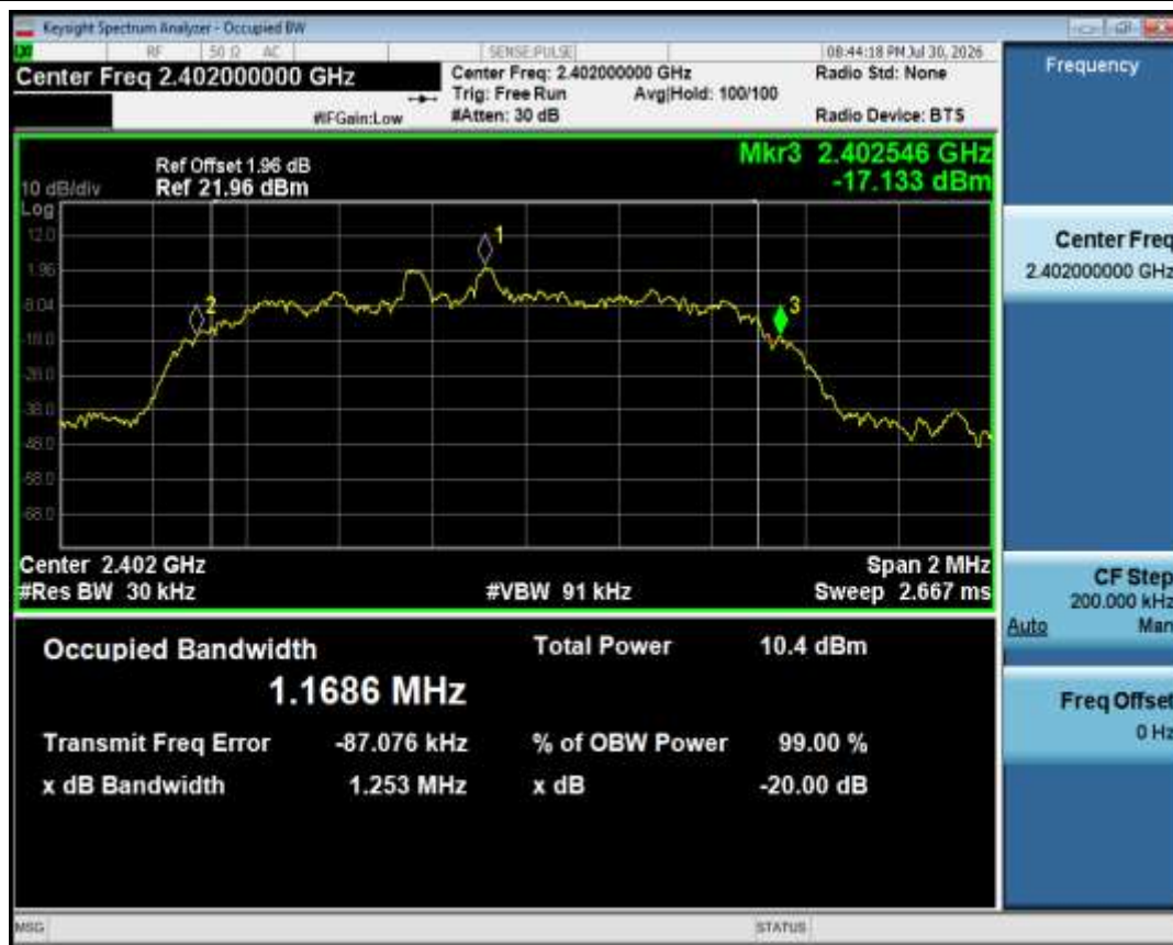
-20dB Bandwidth NVNT 2-DH1 2402MHz Ant1
