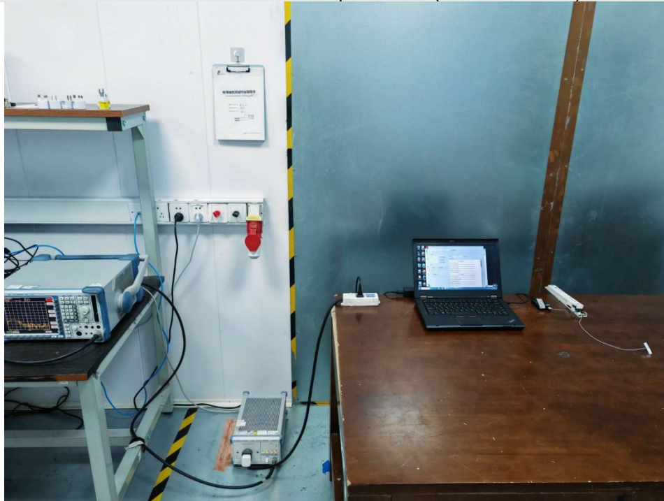
Conducted emissions at AC power line (150kHz-30MHz)
