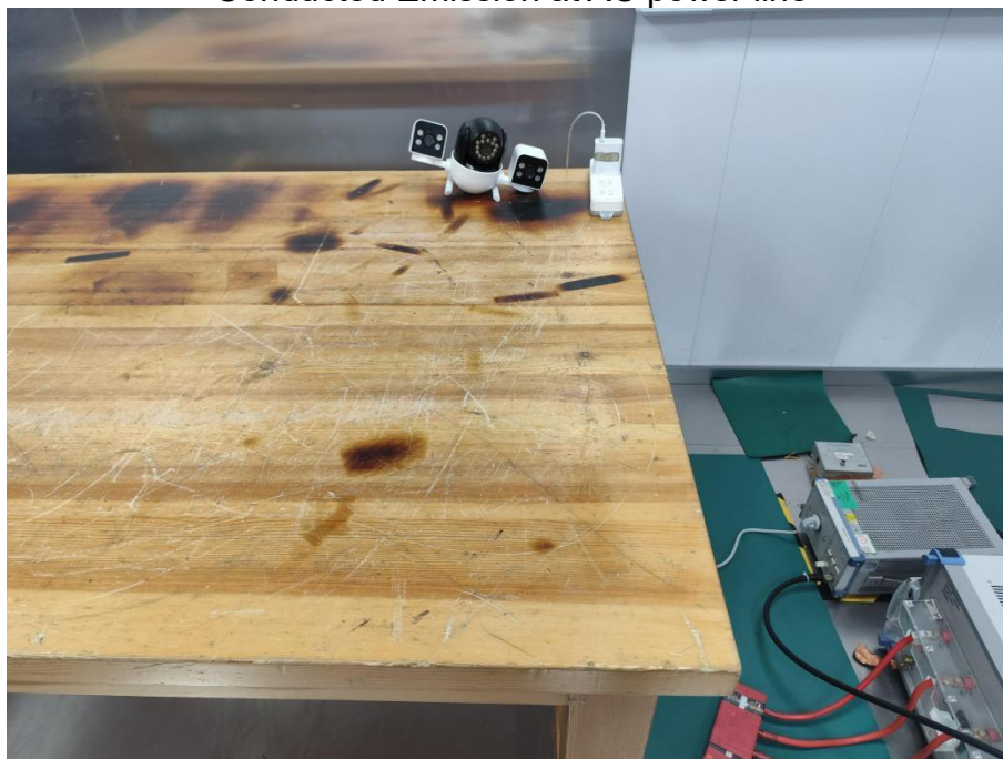
Conducted Emission at AC power line
