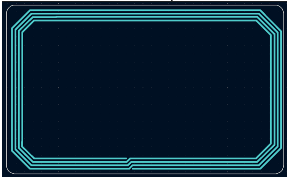
Antenna PCB Layout
