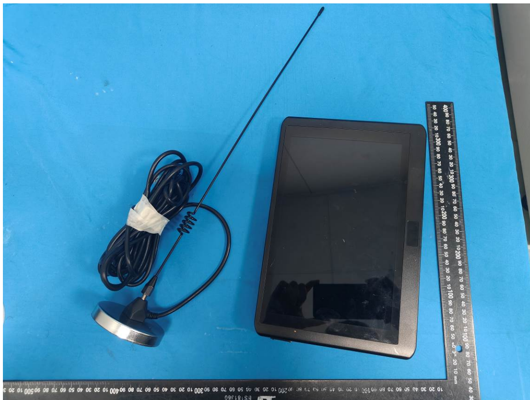
Radio Antenna with Coaxial Harness (For 915MHz Receive Only)
