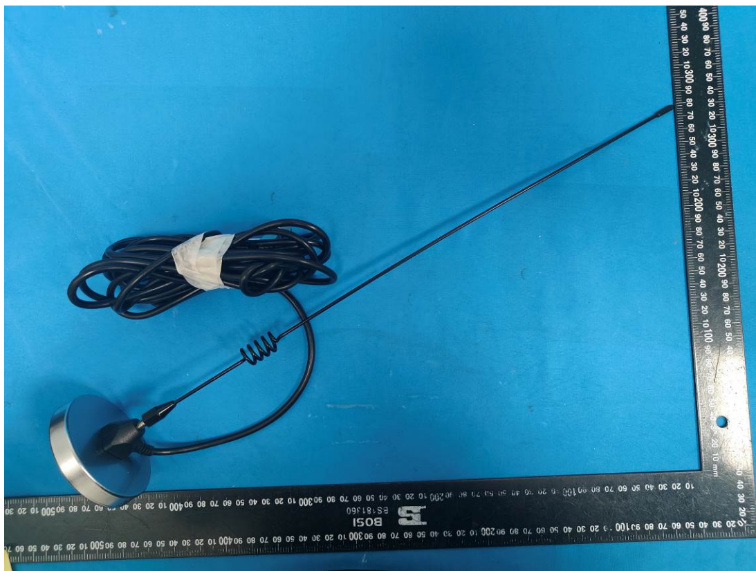
Radio Antenna with Coaxial Harness (For 915MHz Receive Only)
