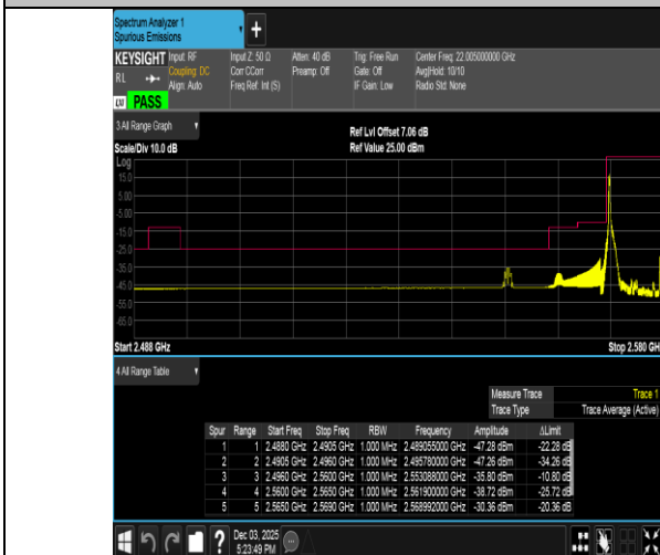
Band38-10MHz-QPSK-37800-1RB#0-PASS
