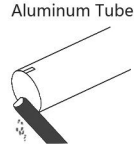
Step 2 Ensure tube edges are clean and free of burrs.
