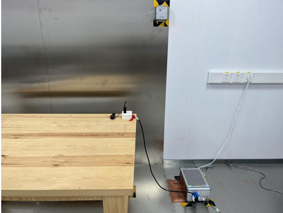
Radiated Emission Test View|(Below 1G)
