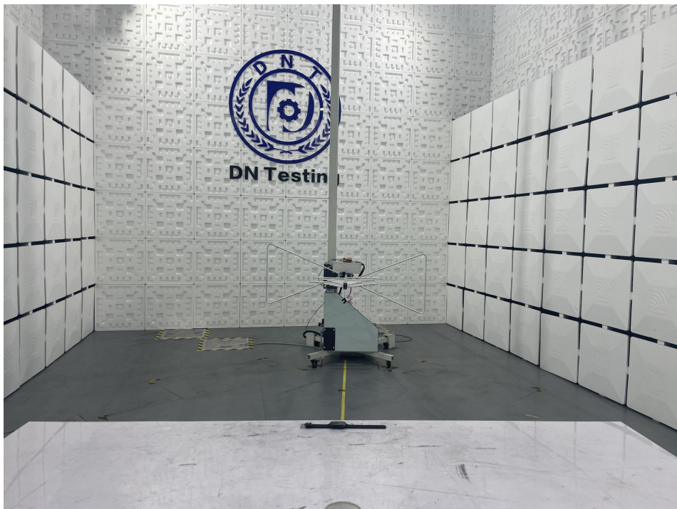
Radiated Emission Test View|(Below 1G)
