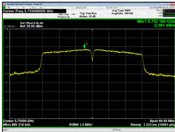
PSD NVNT ac40 5795MHz Ant2
