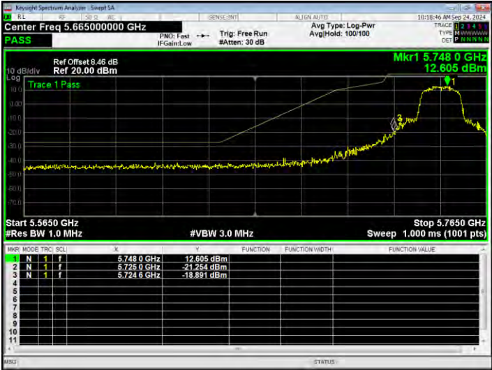
Band Edge NVNT a 5825MHz High Ant2
