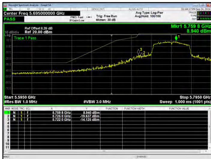
Band Edge NVNT ac40 5795MHz High Ant2
