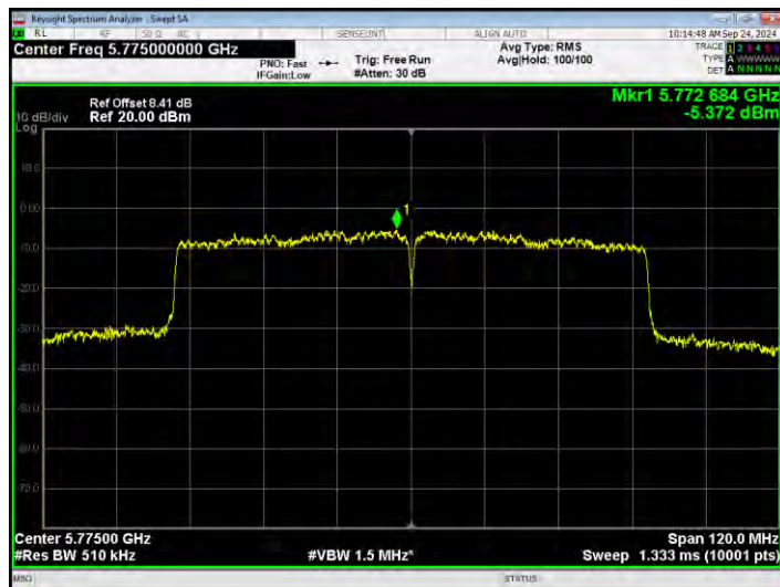
PSD NVNT n20 5745MHz Ant1
