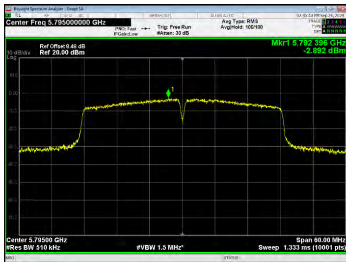
PSD NVNT ac80 5775MHz Ant2
