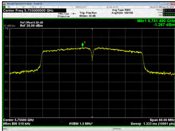
PSD NVNT ax40 5795MHz Ant1
