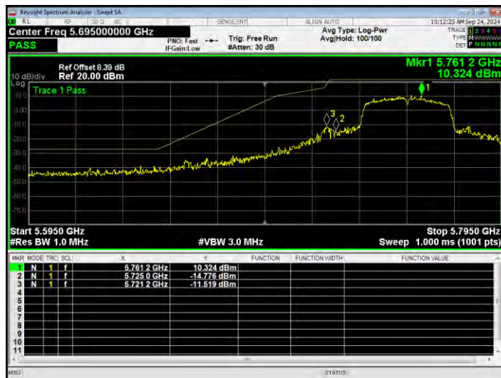
Band Edge NVNT ax40 5795MHz High Ant1
