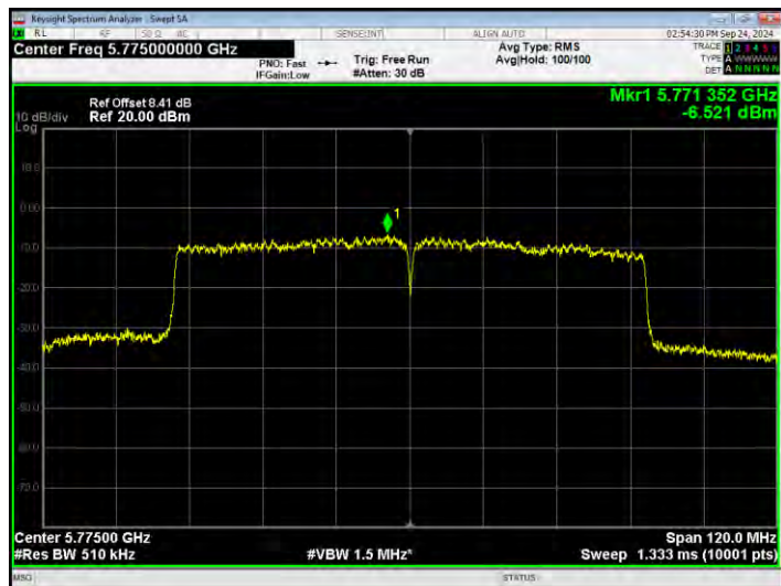
PSD NVNT n20 5745MHz Ant2
