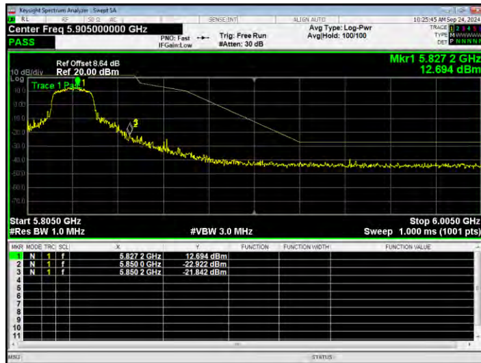
Band Edge NVNT n40 5755MHz Low Ant2
