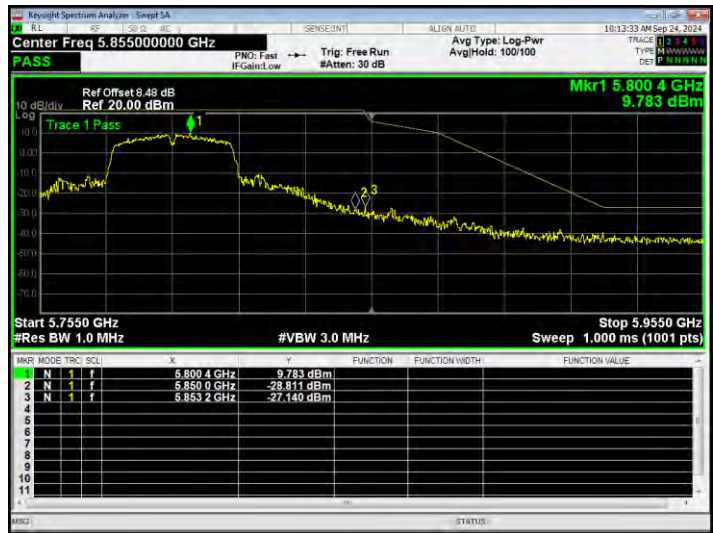
Band Edge NVNT n20 5745MHz Low Ant1
