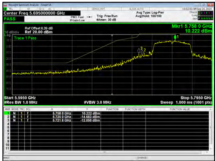
Band Edge NVNT ac40 5795MHz High Ant1
