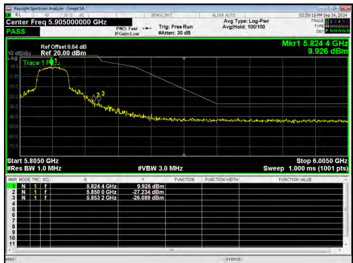
Band Edge NVNT ax40 5755MHz Low Ant2
