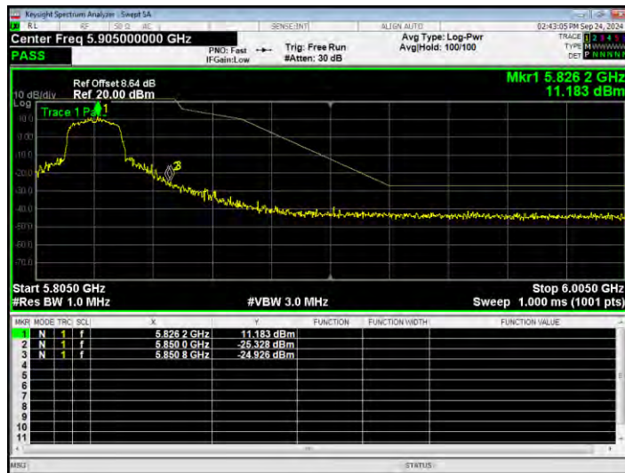
Band Edge NVNT ac40 5755MHz Low Ant2
