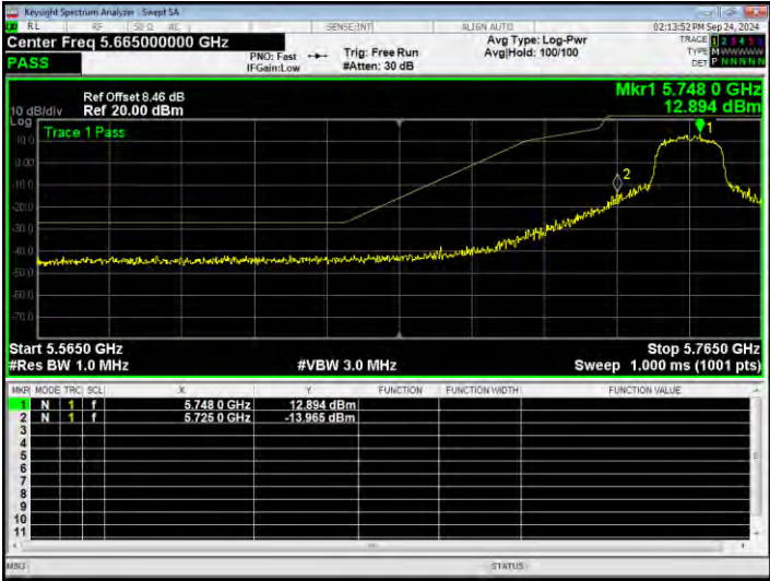
Band Edge NVNT ac20 5785MHz Mid Ant2
