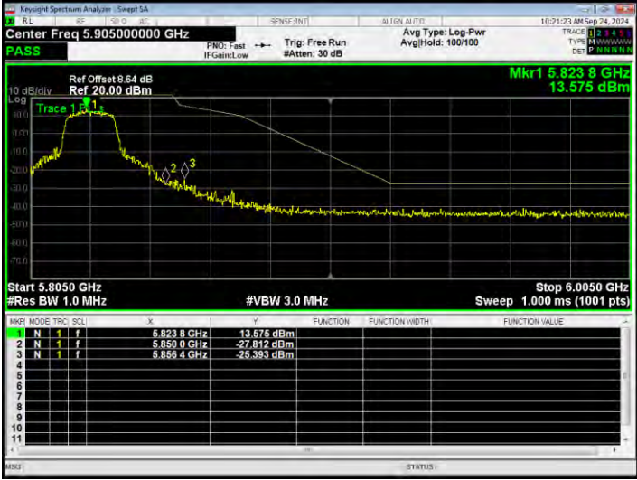
Band Edge NVNT ac20 5745MHz Low Ant2
