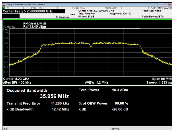
(802.11 ac40) 26dB Bandwidth plot on channel 46
