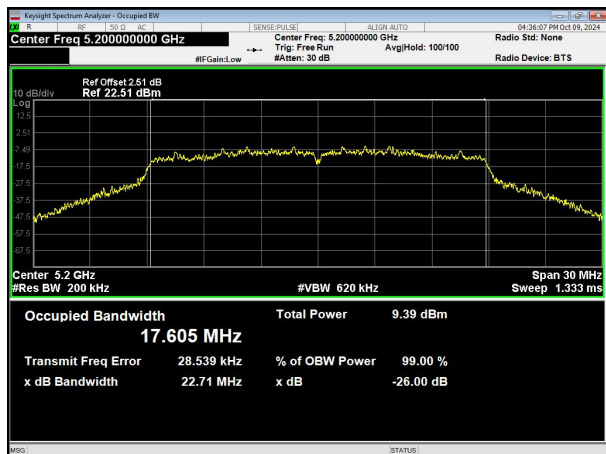
(802.11ac20) 26dB Bandwidth plot on channel 40
