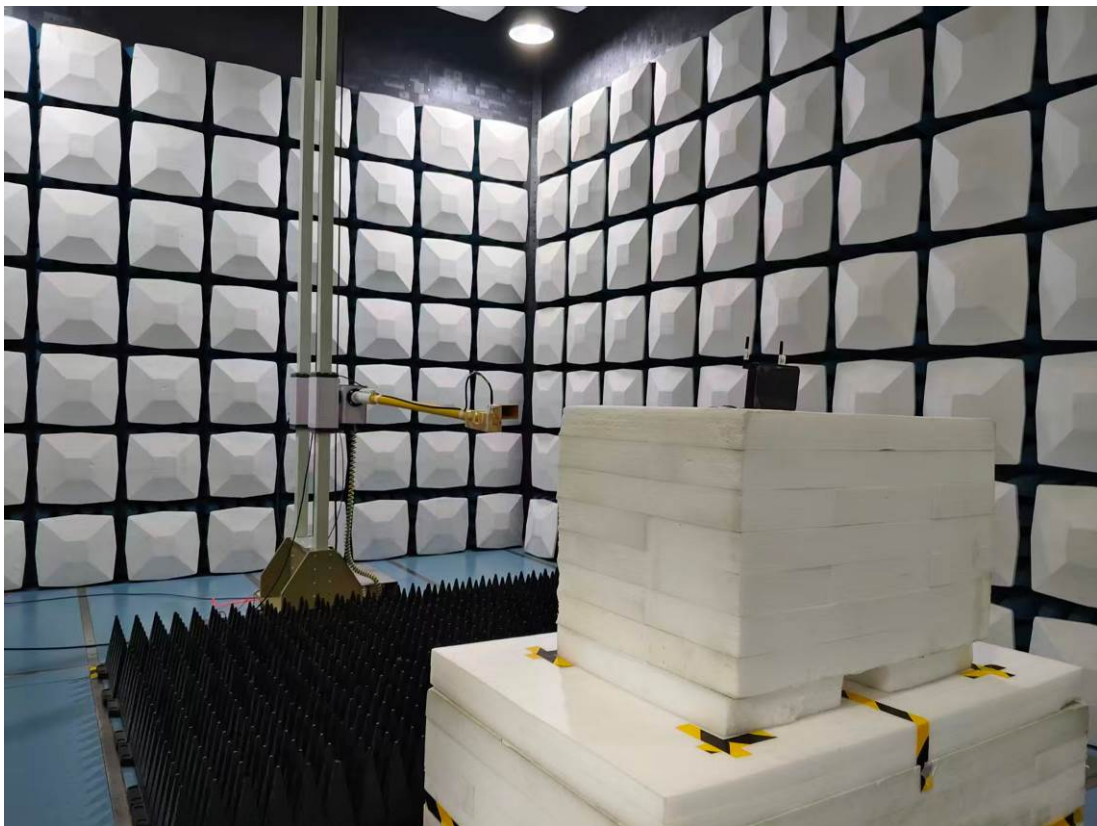
Radiated Emission 18-26.5GHz View
