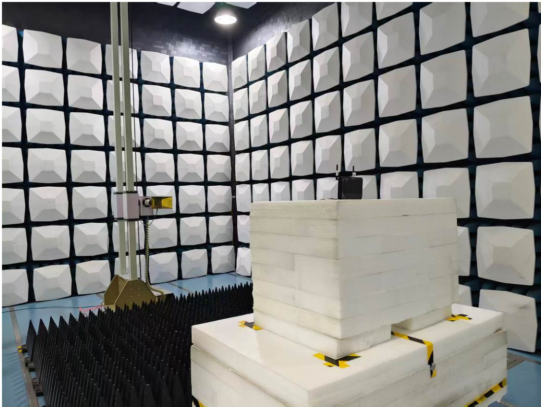
Radiated Emission 18-26.5GHz View
