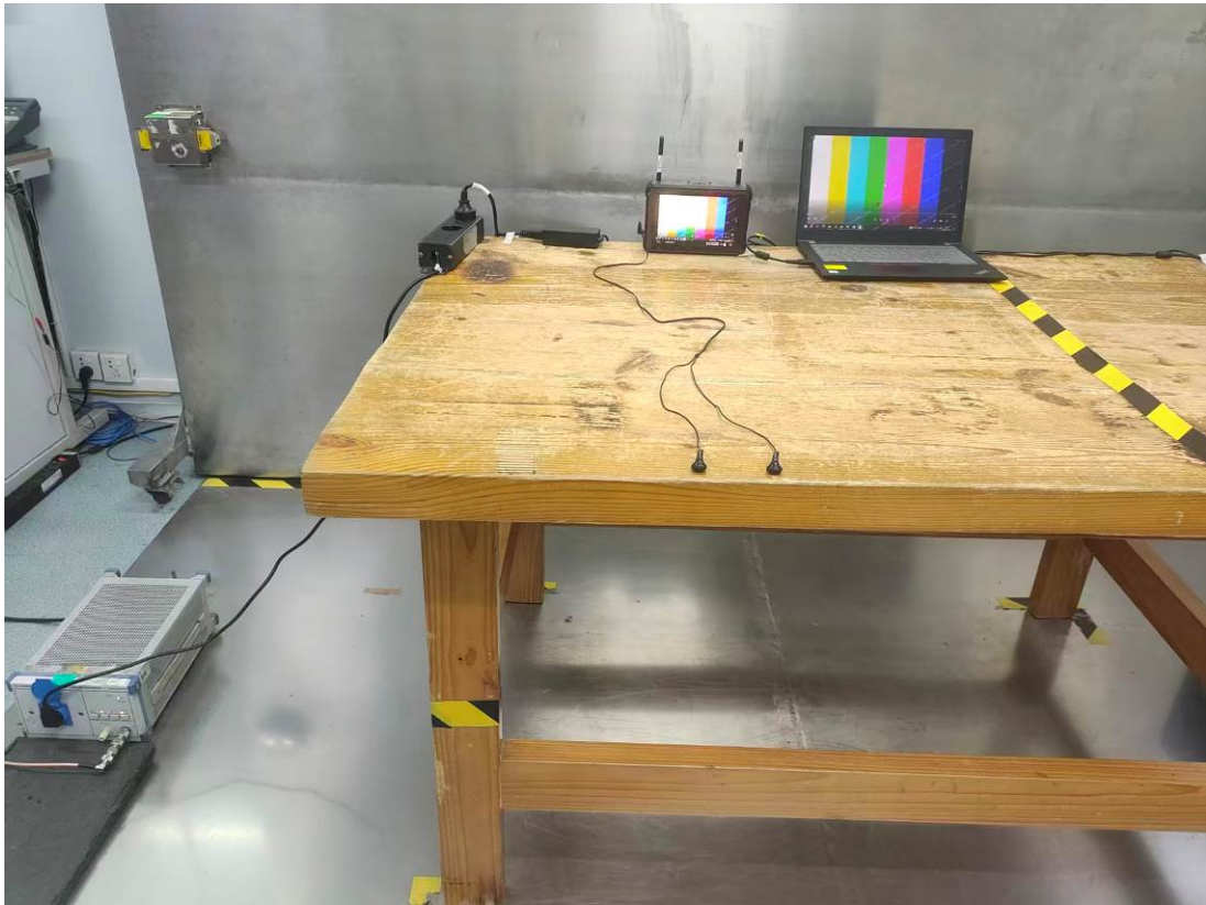
Conducted Emissions Side View
