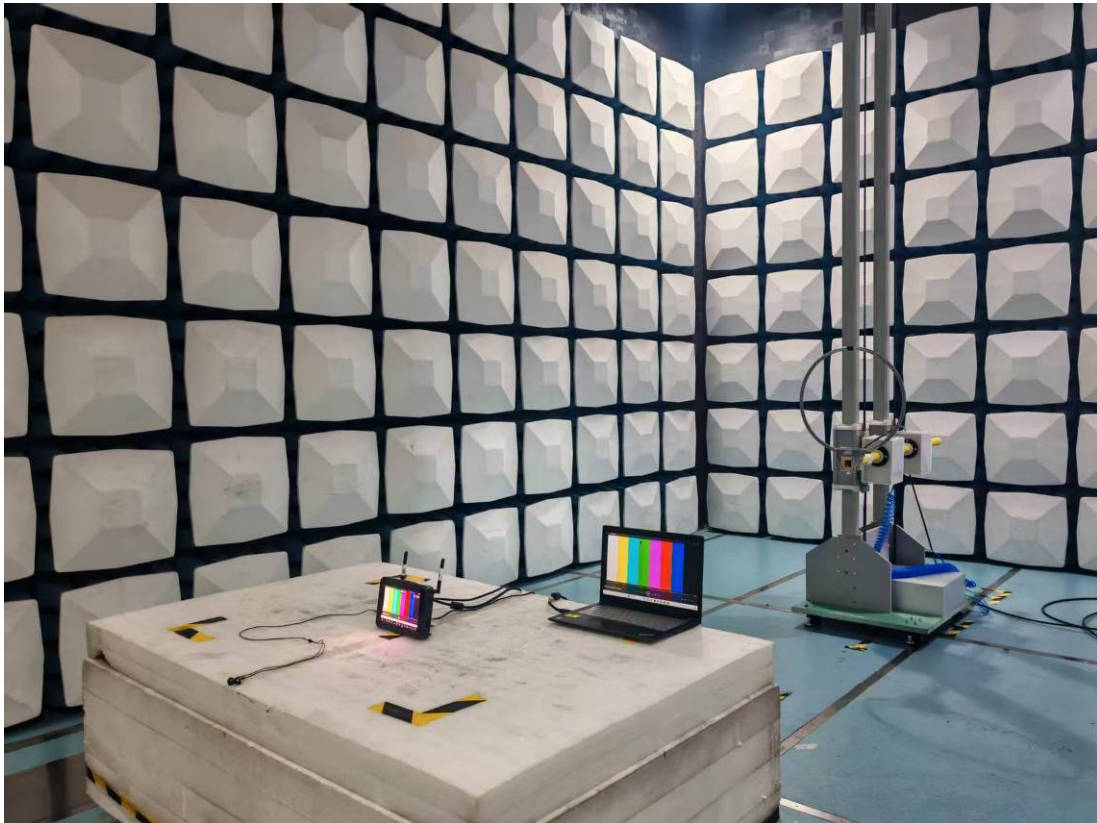
Radiated Emission 9k-30MHz Perpendicular View
