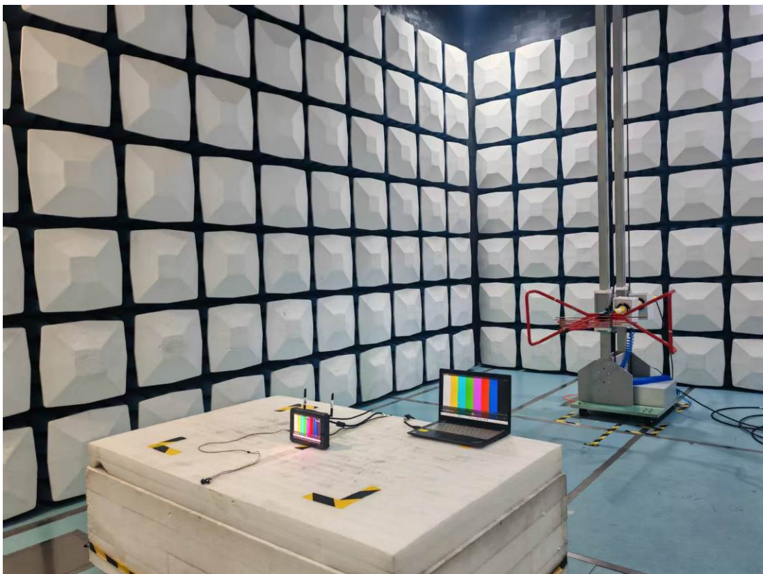
Radiated Emission 30M-1GHz View
