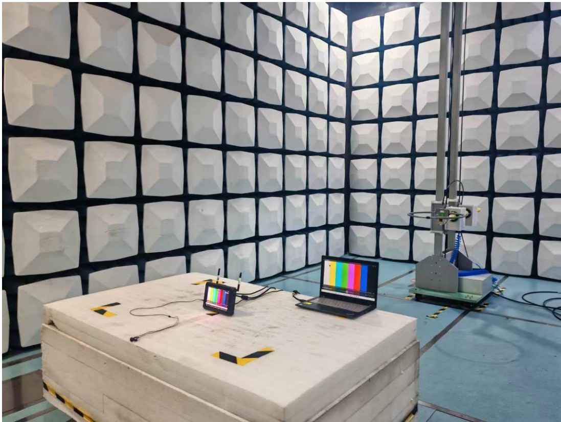
Radiated Emission 30M-1GHz View
