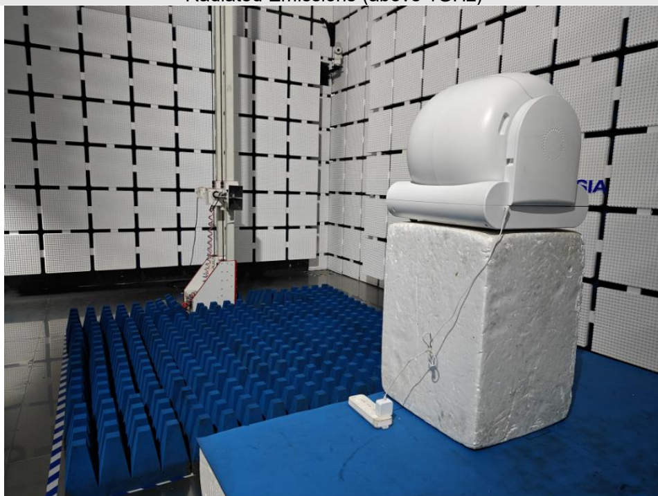
Radiated Emissions (above 1GHz)
