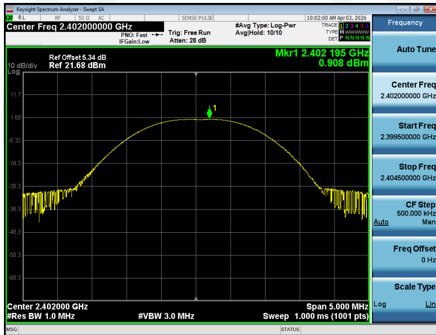
Peak Output Power_NVNT_ANT1_1-DH1_2402_00
