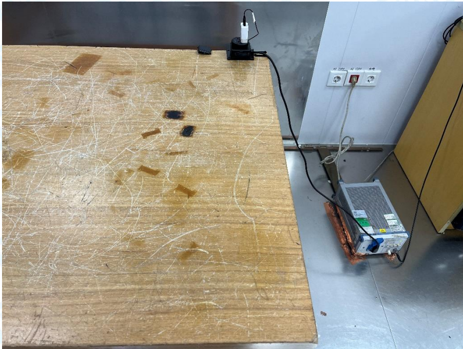
Photo of Setup for Radiated Emission (30MHz~1GHz)
