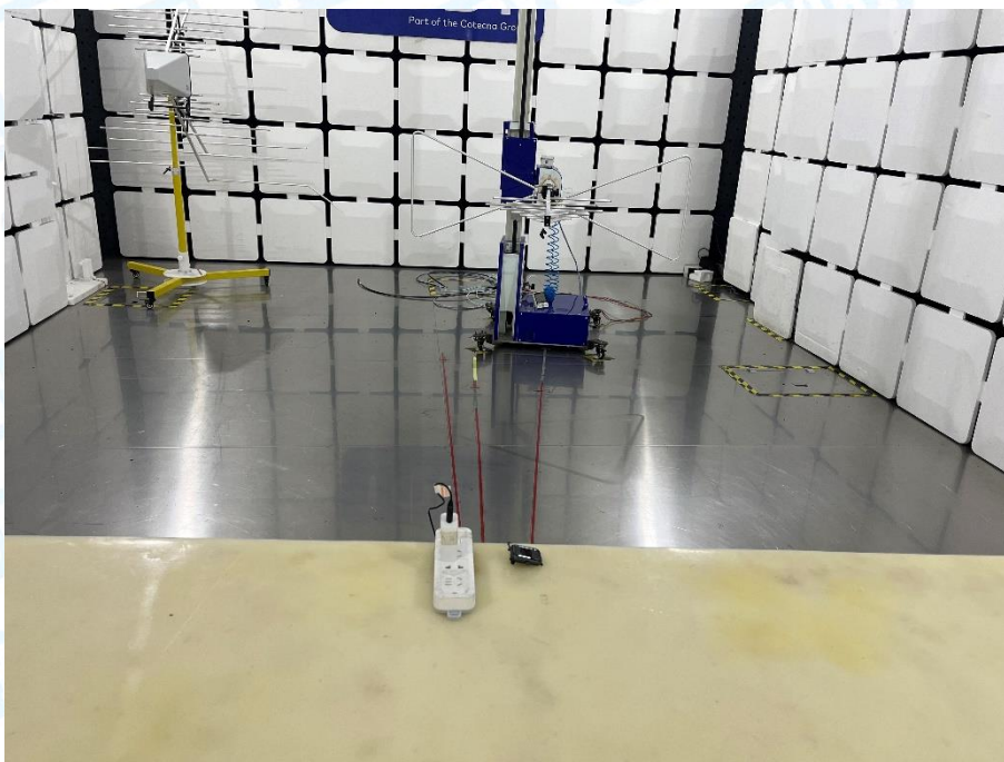
Photo of Setup for Radiated Emission (30MHz~1GHz)
