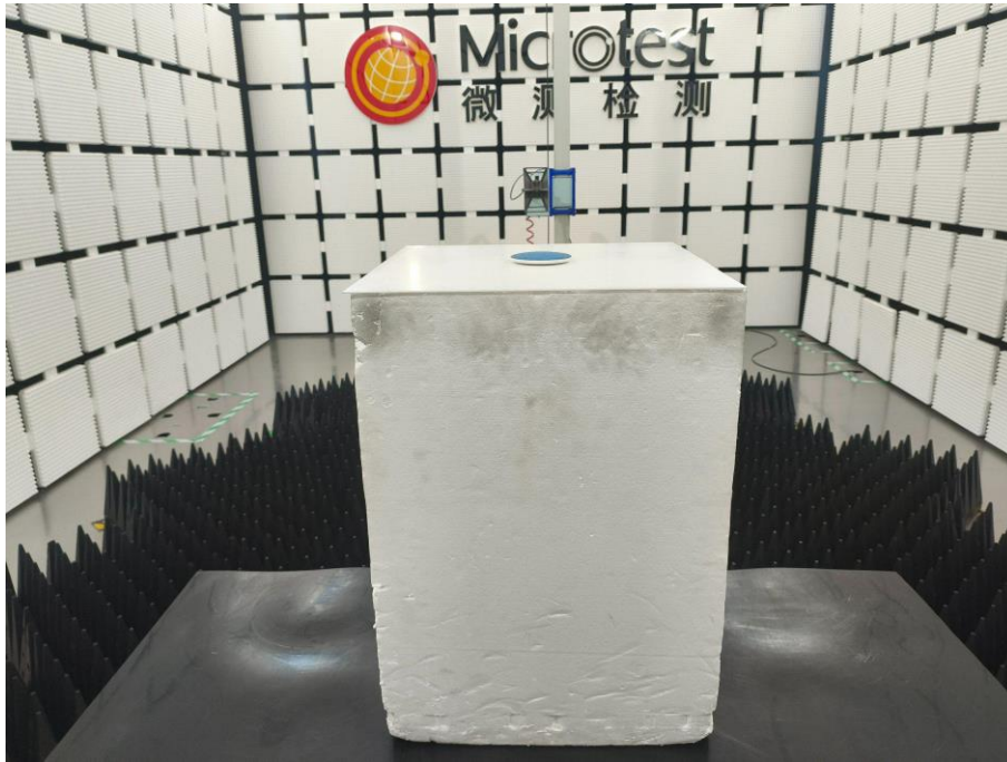
Radiated emissions (above 1GHz)
