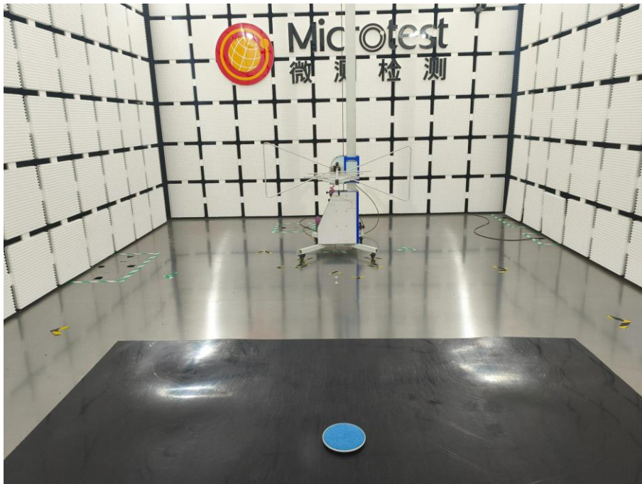
Radiated emissions (below 1GHz)
