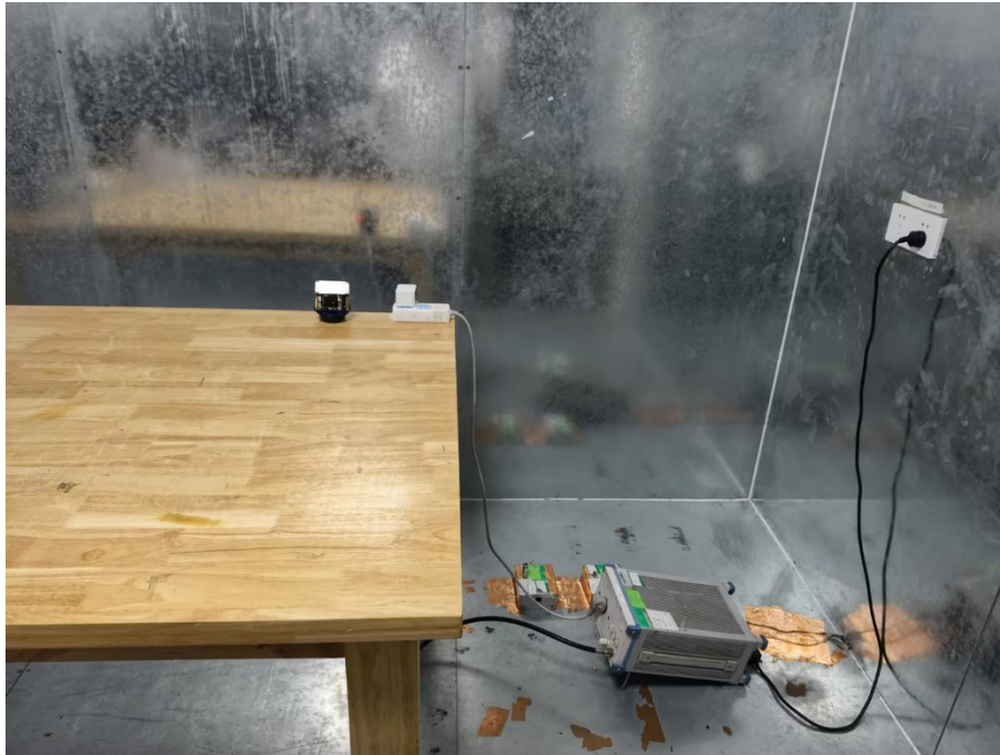
Photograph 3: Set-up photo for AC Power Conducted Emission
