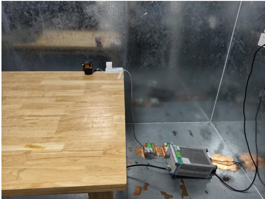
Photograph 3: Set-up photo for AC Power Conducted Emission
