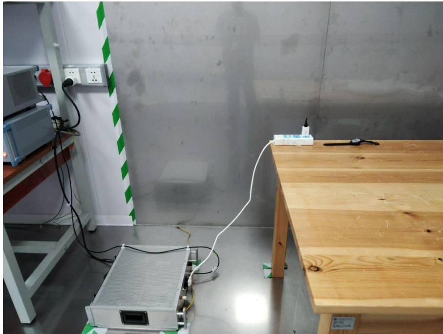
Conducted Emission at AC power line
