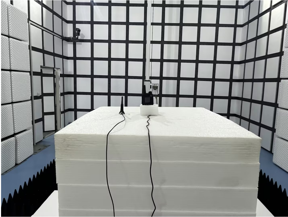
Radiation Emission - Back View (Above 18GHz)
