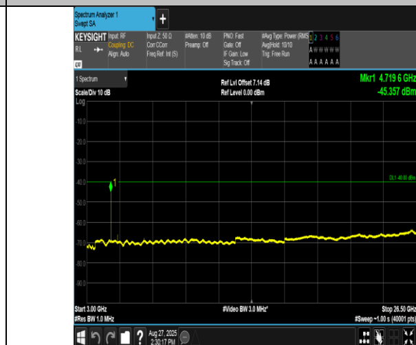
Band40(2350-2360)-5MHz-QPSK-39225-1RB#24-3000~26500-PASS
