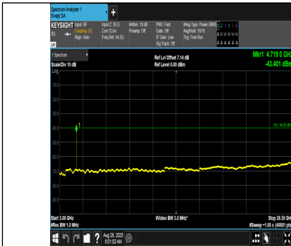
Band40(2350-2360)-10MHz-QPSK-39200-1RB#49-3000~26500-PASS
