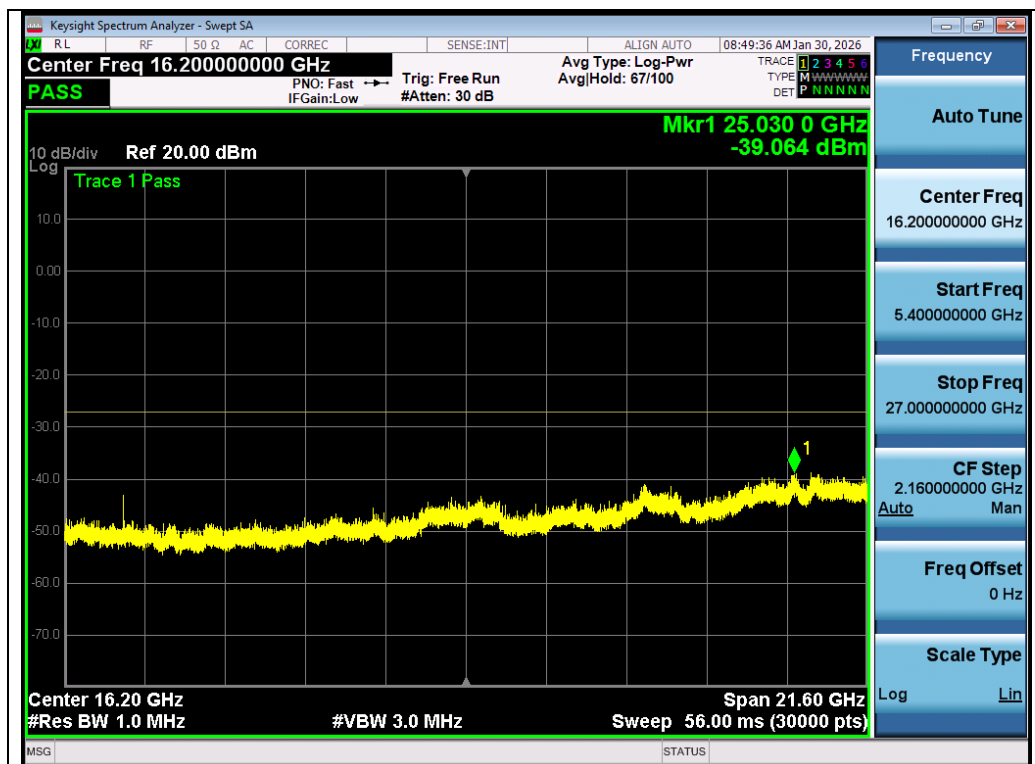
Test_Graph_802.11a_Chain A_5240_6Mbps_Frequency Band 4
