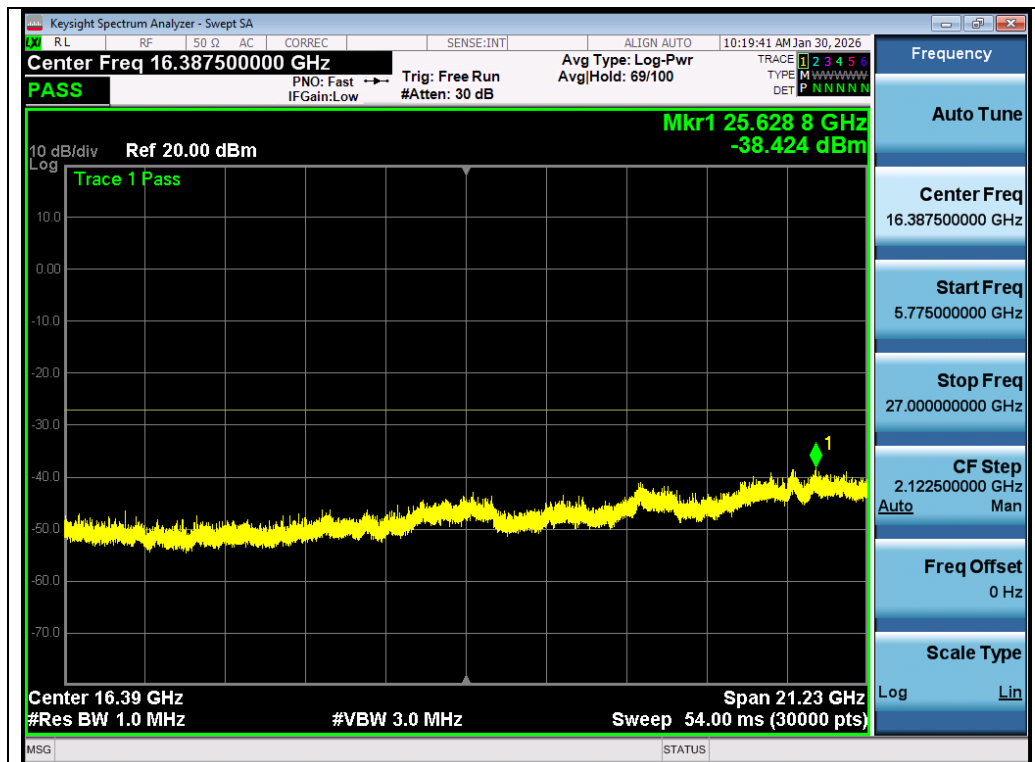
Test_Graph_802.11ac80_Chain A_5530_MCS0_Frequency Band 4
