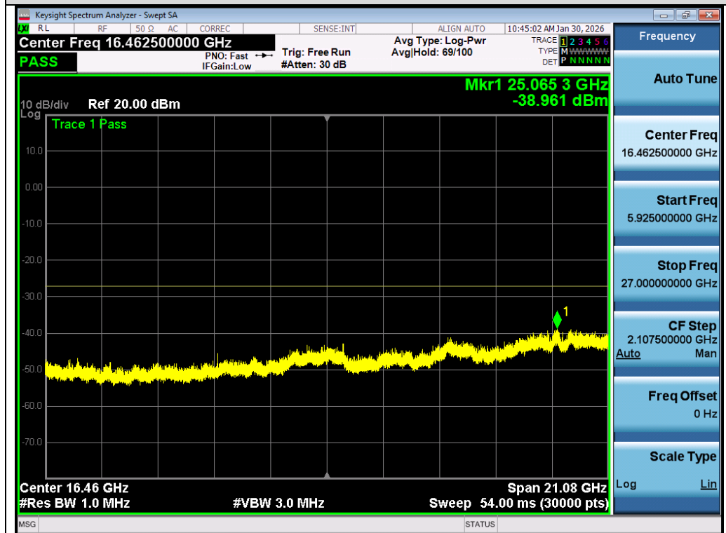
Test_Graph_802.11n40_Chain A_5795_MCS0_Frequency Band4
