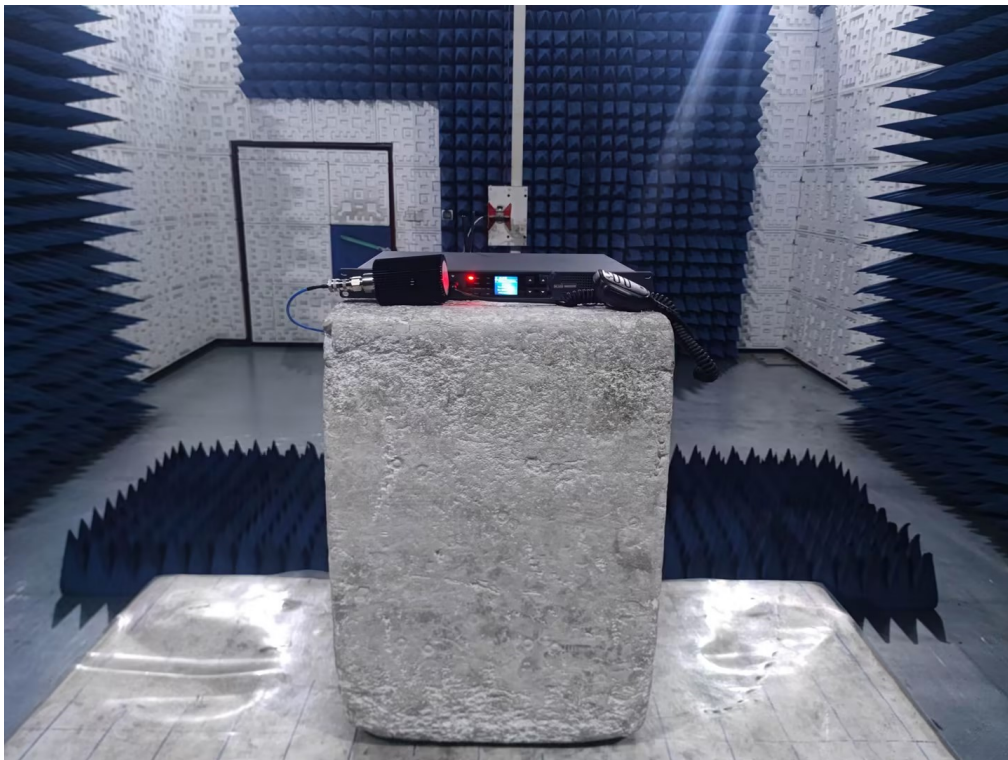
Radiated Emission Test Setup Above 1GHz
