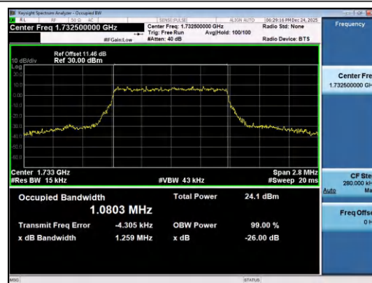
Band4-1.4MHz-16QAM-20175-6RB#0-PASS
