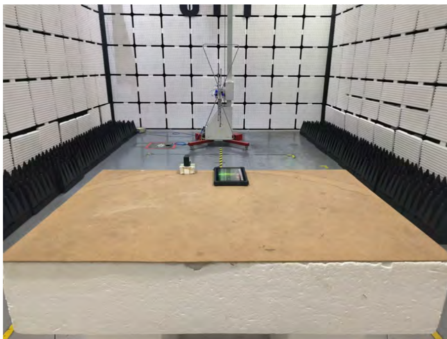
Radiated spurious emission Test Setup-1(Below 1GHz)
