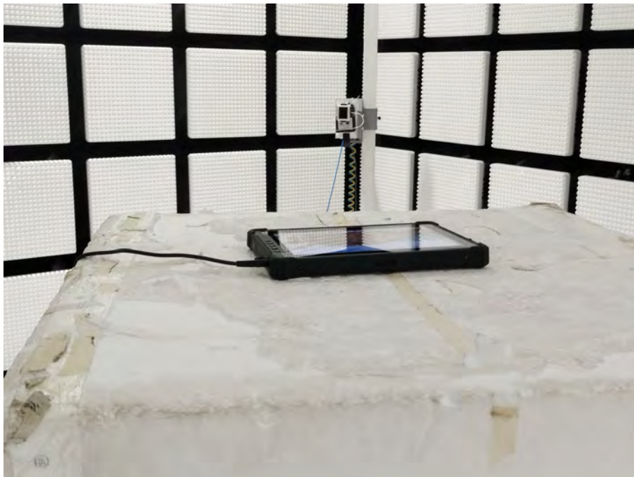
Radiated spurious emission Test Setup-3(Above 18GHz)
