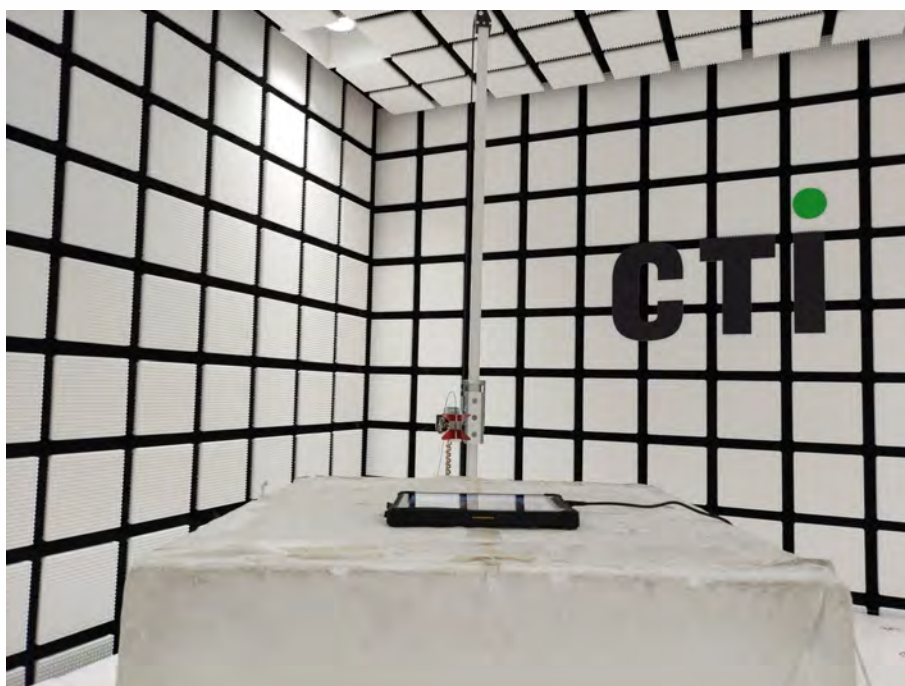
Radiated spurious emission Test Setup-2(Above 1GHz)
