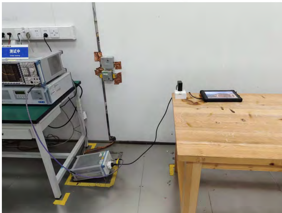
Conducted Emissions Test Setup
