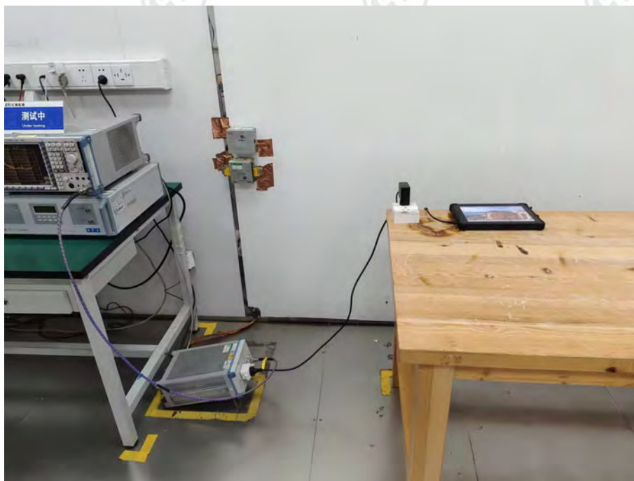
Conducted Emissions Test Setup
