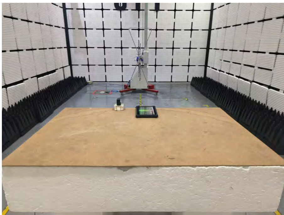
Radiated spurious emission Test Setup-1(Below 1GHz)
