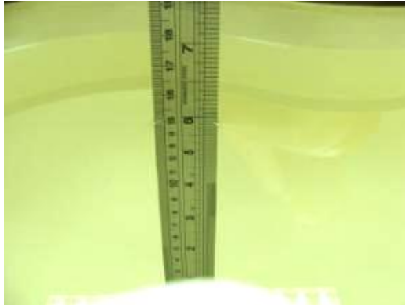
Photo of Liquid Height for Head SAR
