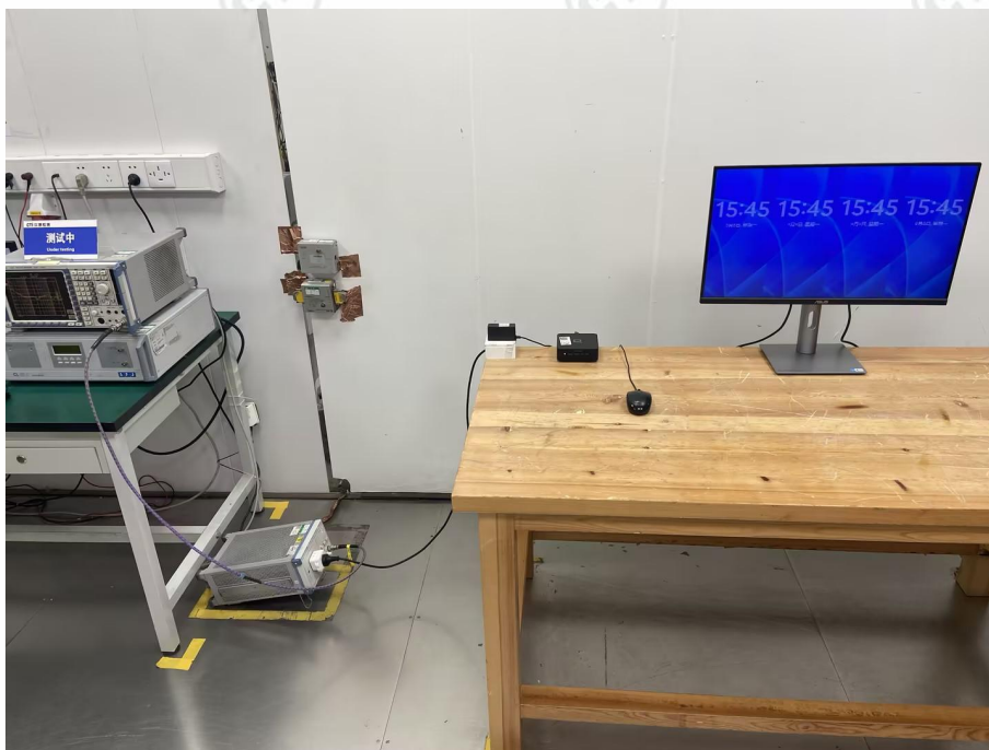
Conducted Emissions Test Setup
