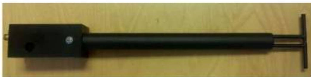
Figure 1 – MVG COMOSAR Validation Dipole
