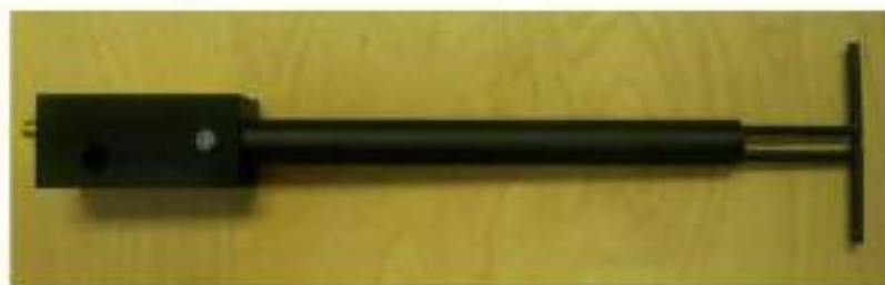
Figure 1 – MVG COMOSAR Validation Dipole
