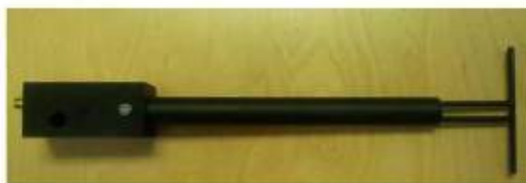
Figure 1 – MVG COMOSAR Validation Dipole
