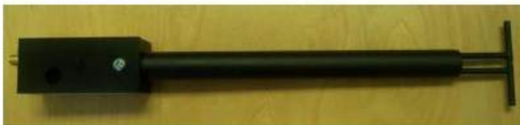
Figure 1 – MVG COMOSAR Validation Dipole
