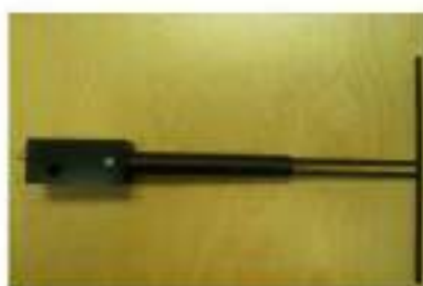
Figure 1 – MVG COMOSAR Validation Dipole
