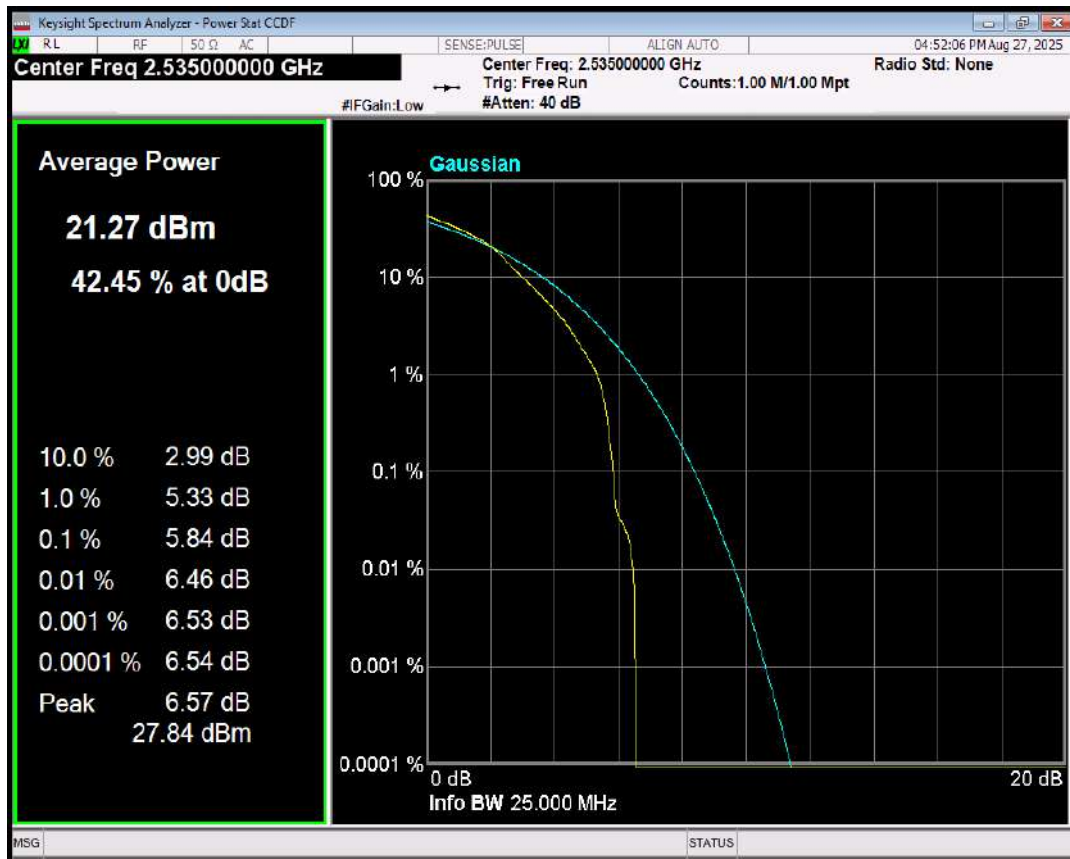
Band7 QPSK BW=10MHz Channel=21100 RB Size=1 Position=#0
