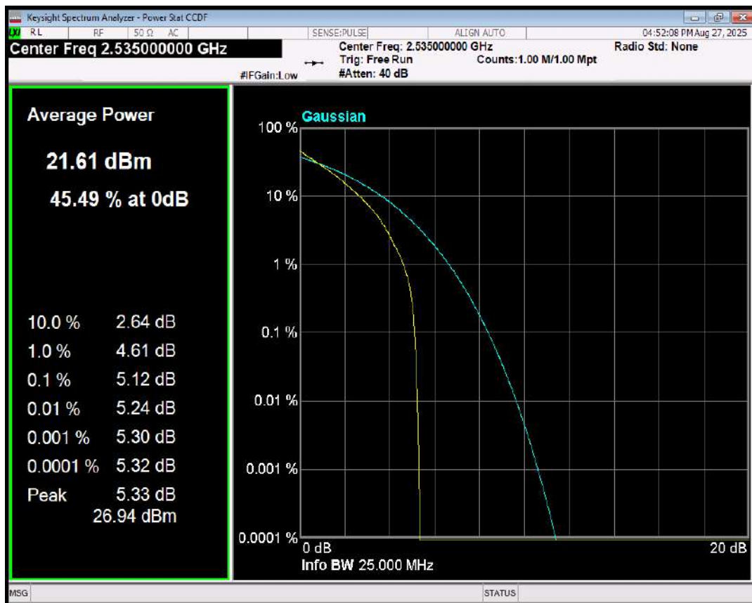
Band7 16QAM BW=10MHz Channel=21100 RB Size=1 Position=#0
