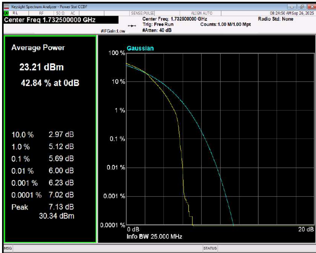
Band7 QPSK BW=5MHz Channel=21100 RB Size=1 Position=#0
