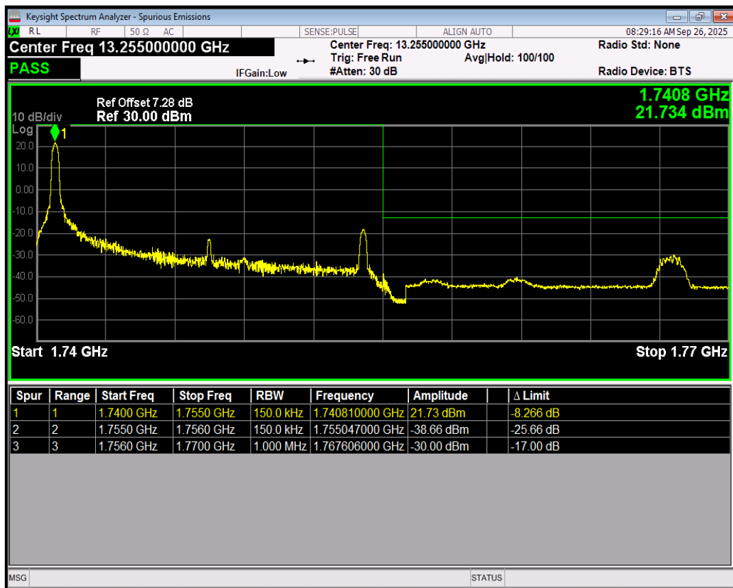
Band4 16QAM BW=15MHz Channel=20325 RB Size=1 Position=#Max
