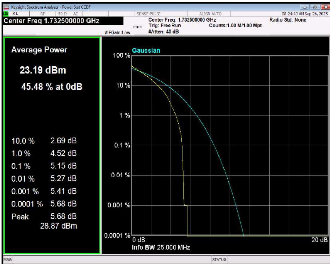
Band4 16QAM BW=15MHz Channel=20175 RB Size=1 Position=#0
