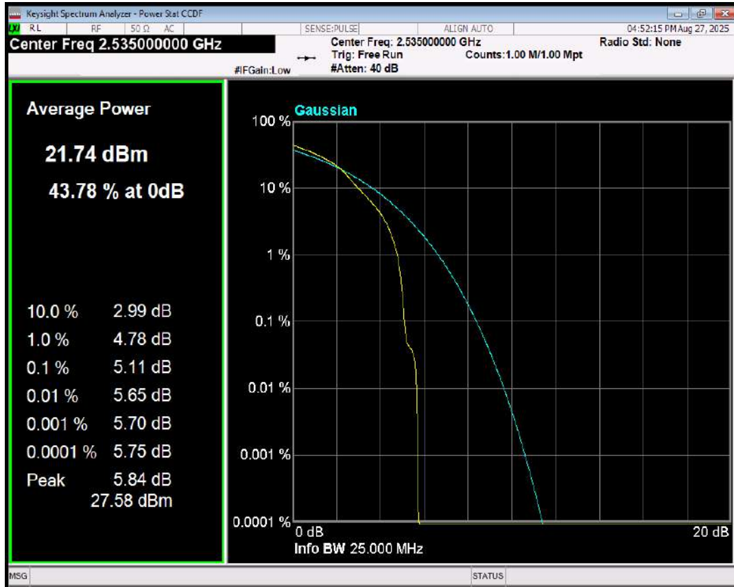
Band7 QPSK BW=20MHz Channel=21100 RB Size=1 Position=#0
