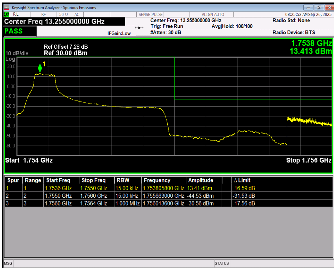
Band4 16QAM BW=1.4MHz Channel=20393 RB Size=1 Position=#Max
