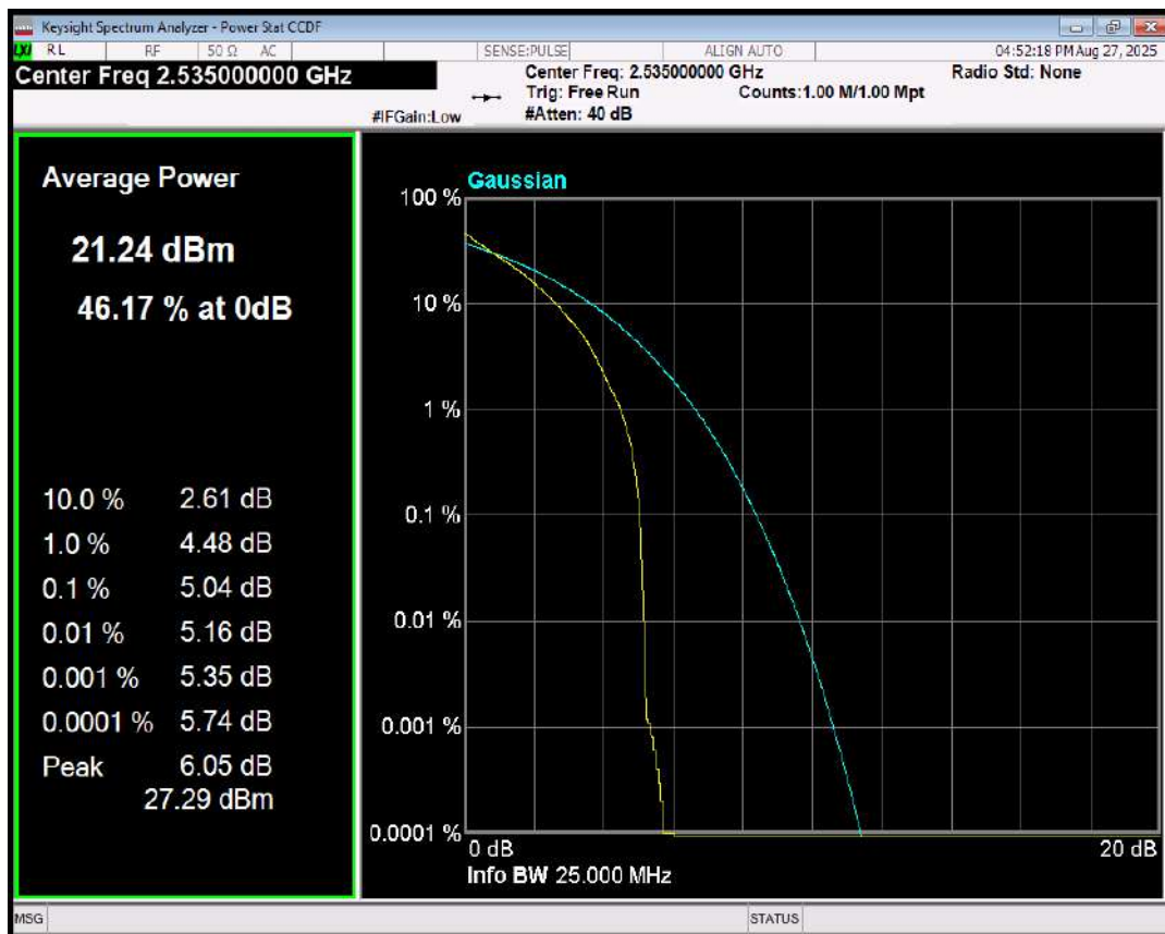
Band7 16QAM BW=20MHz Channel=21100 RB Size=1 Position=#0
