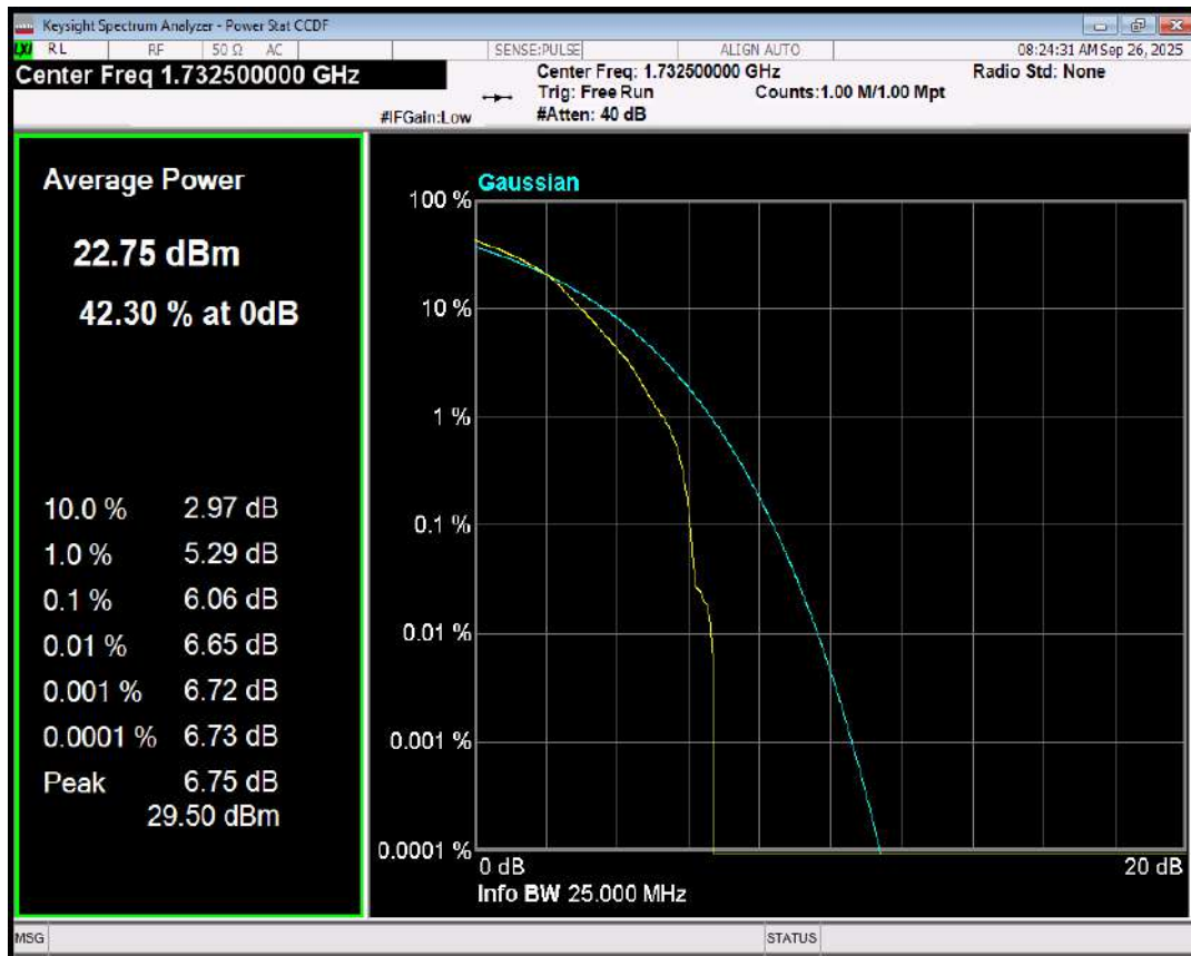
Band4 QPSK BW=5MHz Channel=20175 RB Size=1 Position=#0
