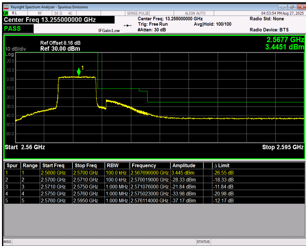
Band7 QPSK BW=10MHz Channel=20800 RB Size=1 Position=#0
