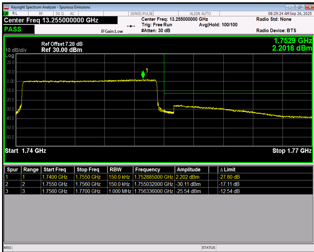
Band4 QPSK BW=20MHz Channel=20050 RB Size=1 Position=#0
