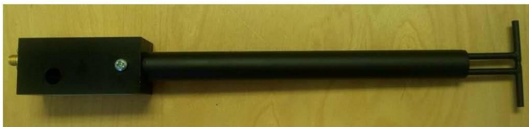
Figure 1 – MVG COMOSAR Validation Dipole
