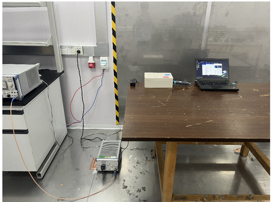
Conducted Emission Test Setup
