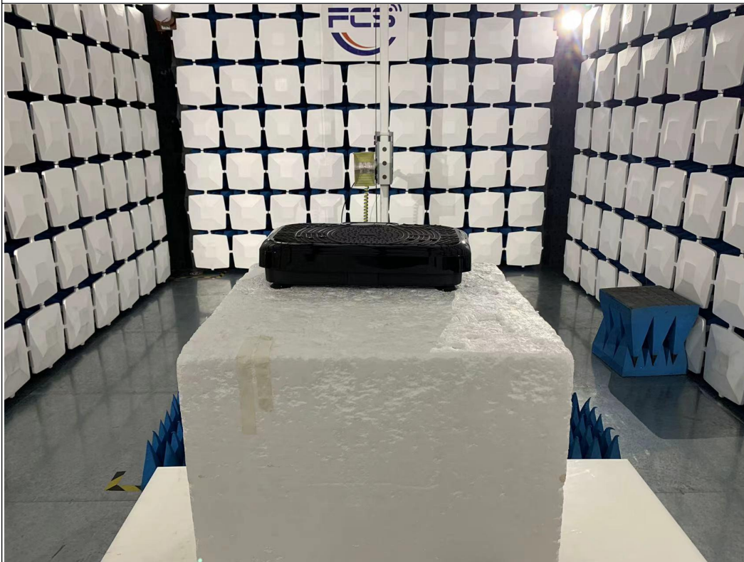
Above 1GHz for radiated emission test setup
