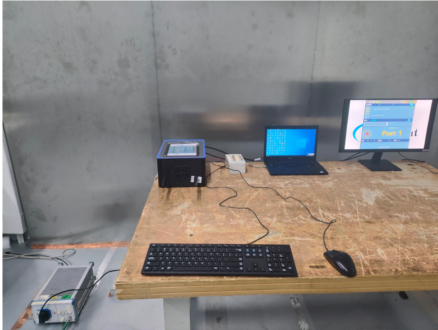
Conducted Emissions - Side View
