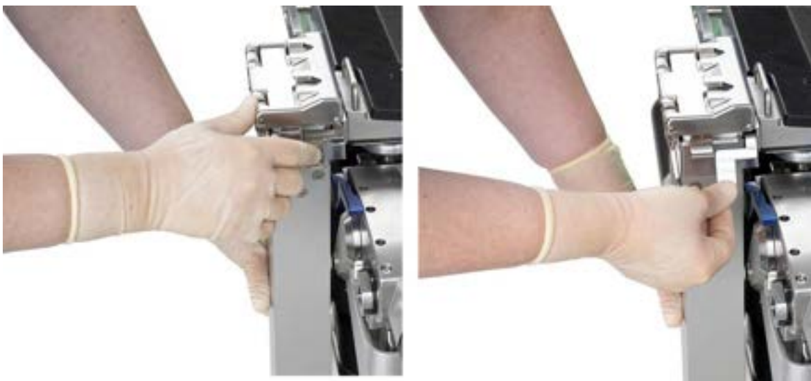
Figure 76: Raising the Locking Lever on the Femur Lift
