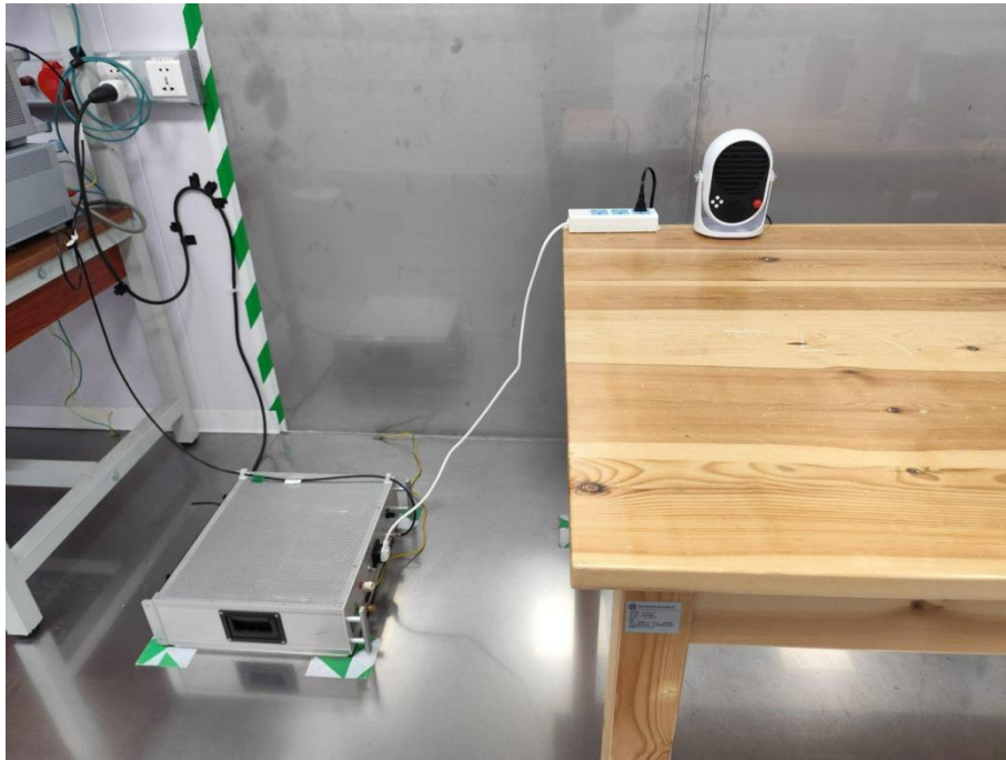
Conducted Emission at AC power line
