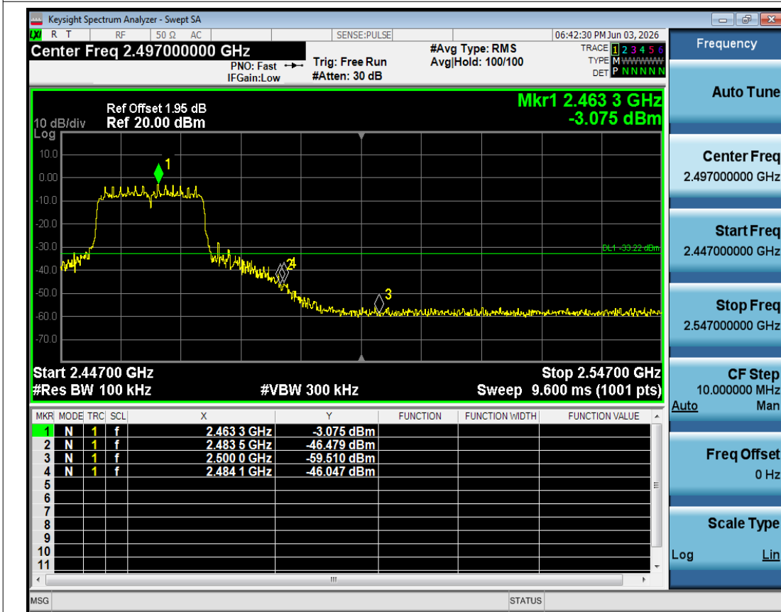
Band Edge NVNT n20 2462MHz Ant1 Emission
