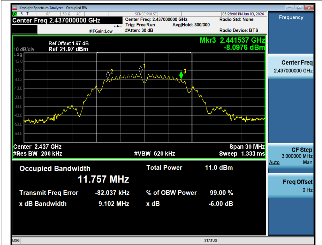
-6dB Bandwidth NVNT b 2437MHz Ant1
