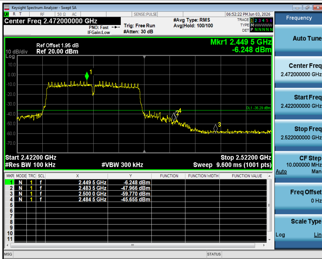
Band Edge NVNT n40 2452MHz Ant1 Emission
