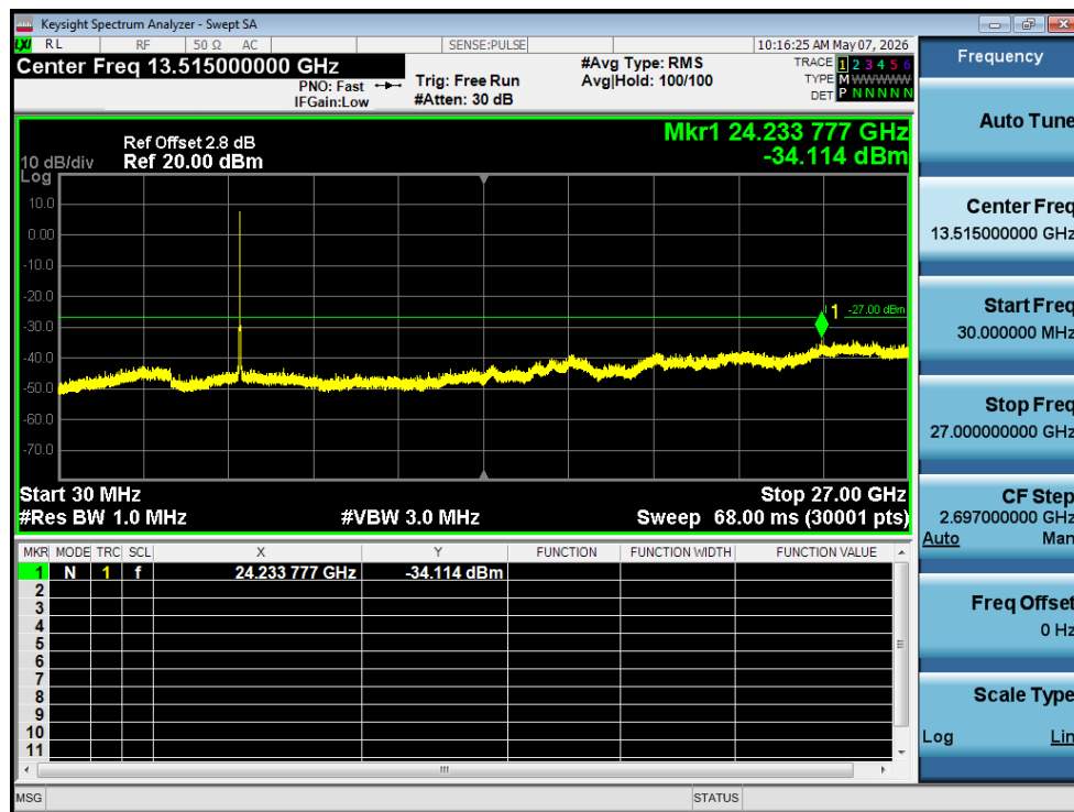
Tx. Spurious NVNT a 5785MHz Ant1 Emission
