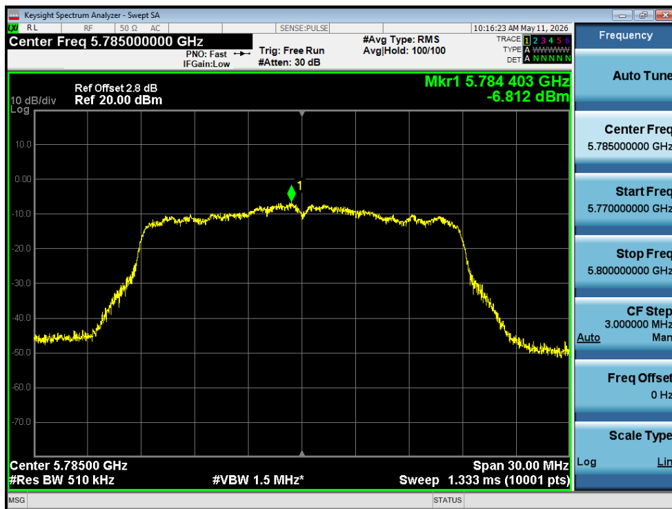
PSD NVNT ac20 5785MHz Ant1
