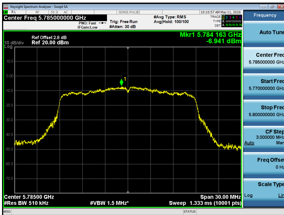
PSD NVNT n20 5785MHz Ant1
