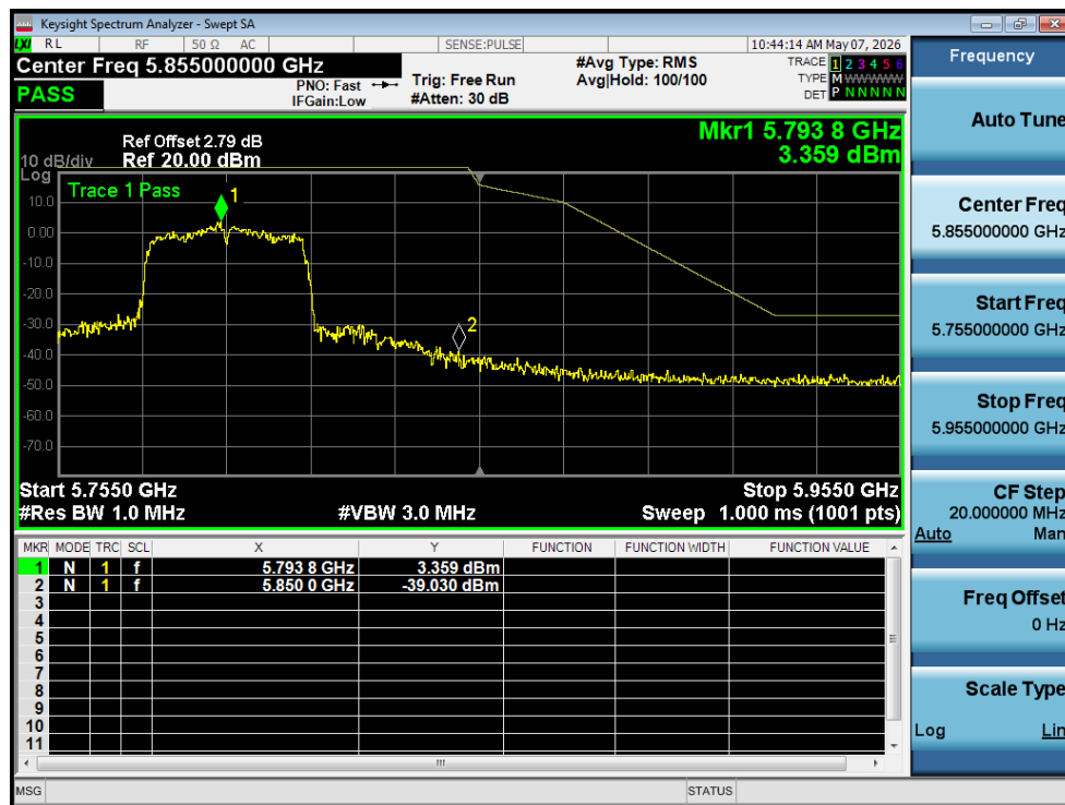
Band Edge NVNT ac40 5795MHz High Ant1
