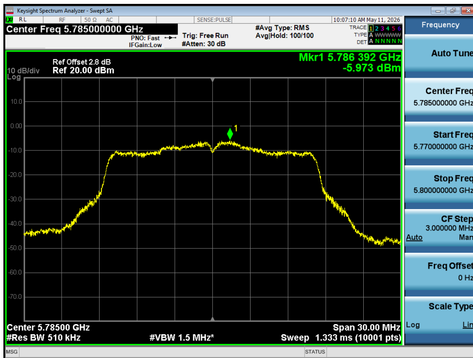
PSD NVNT a 5785MHz Ant1
