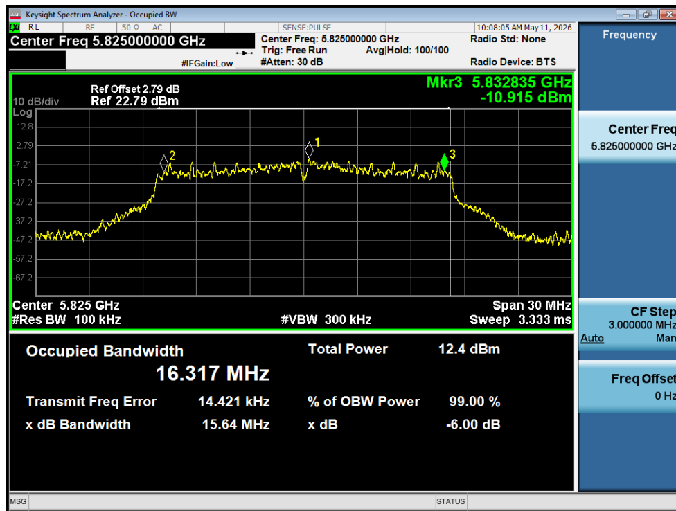
-6dB Bandwidth NVNT a 5825MHz Ant1
