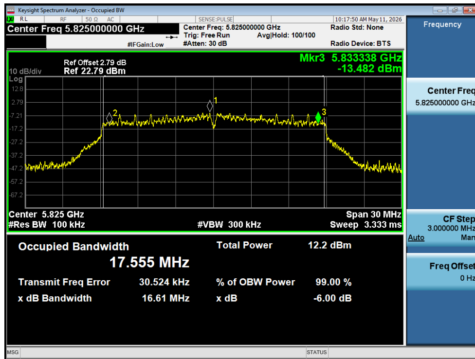
-6dB Bandwidth NVNT ac20 5825MHz Ant1
