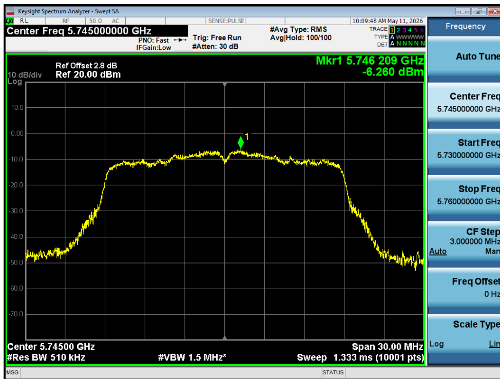
PSD NVNT n20 5745MHz Ant1
