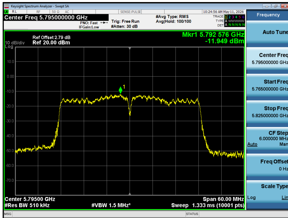
PSD NVNT ac40 5795MHz Ant1
