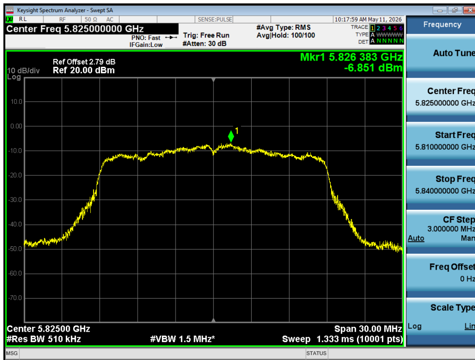
PSD NVNT ac20 5825MHz Ant1
