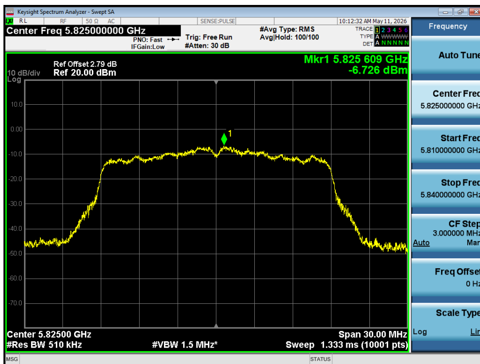
PSD NVNT n20 5825MHz Ant1
