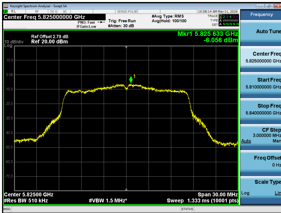
PSD NVNT a 5825MHz Ant1
