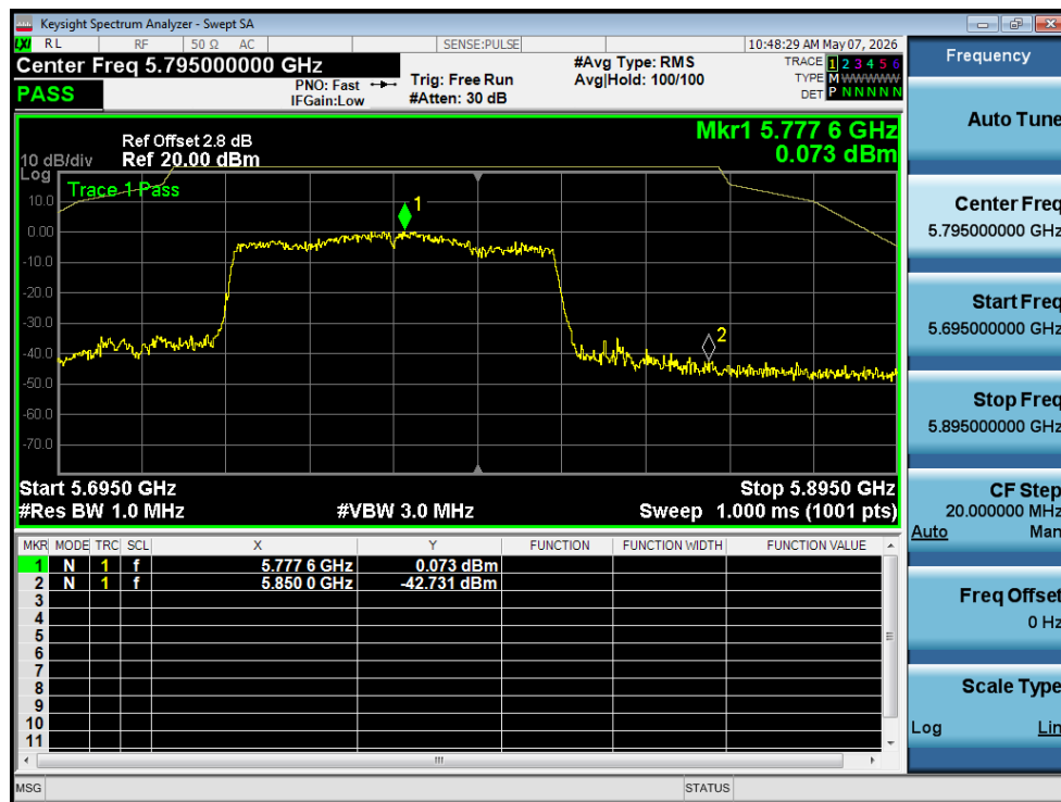
Band Edge NVNT ac80 5775MHz High Ant1
