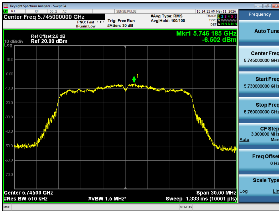
PSD NVNT ac20 5745MHz Ant1
