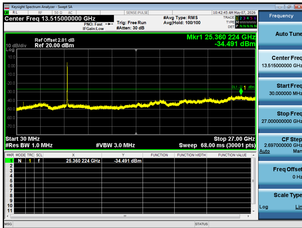
Tx. Spurious NVNT ac40 5755MHz Ant1 Emission
