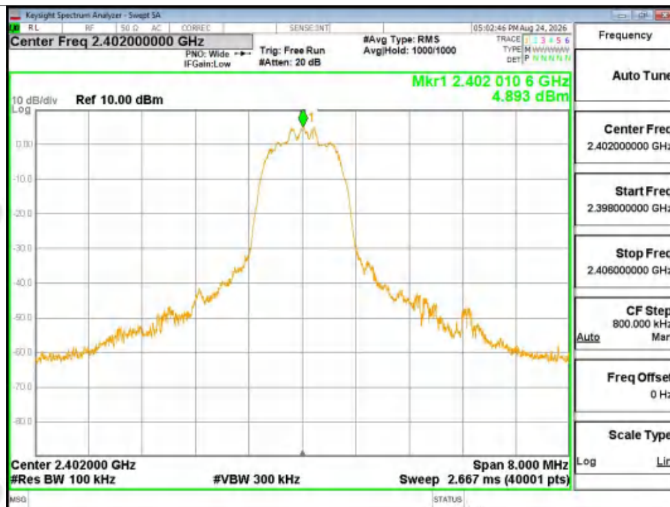
Tx. Spurious NVNT 3-DH5 2402MHz Ant1 Ref
