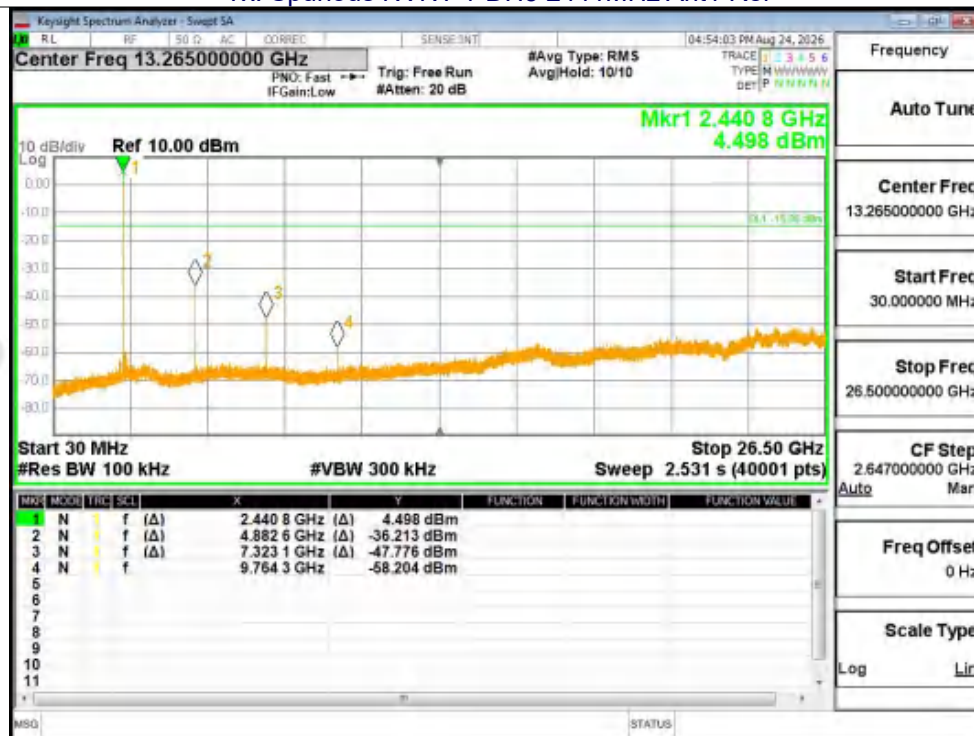
Tx. Spurious NVNT 1-DH5 2441MHz Ant1 Emission
