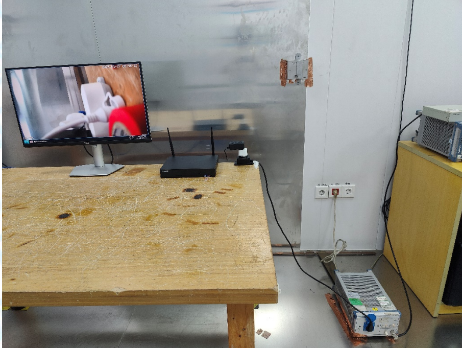
Photo of Setup for Radiated Emission (30MHz~1GHz)
