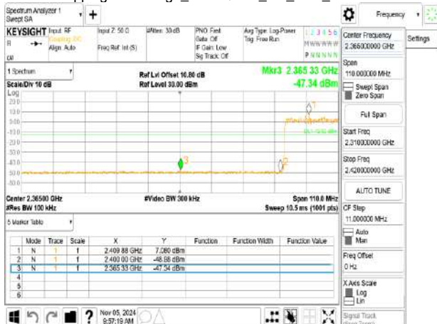
Hopping Band Edge_π/4DQPSK_2M_DH5_2402MHz
