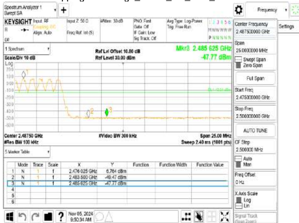
Hopping Band Edge_π/4DQPSK_2M_DH5_2402MHz
