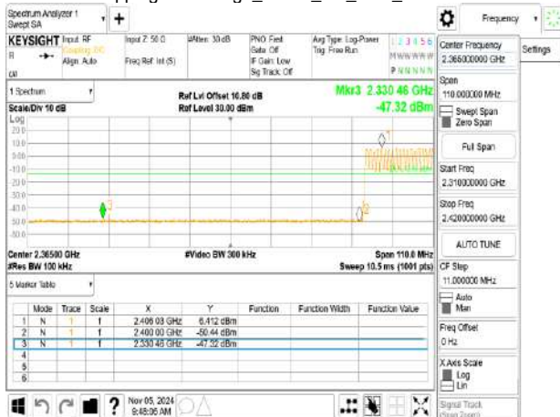
Hopping Band Edge_GFSK_1M_DH5_2480MHz
