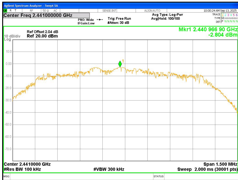
Tx. Spurious NVNT 3-DH1 2441MHz Ant1 Emission
