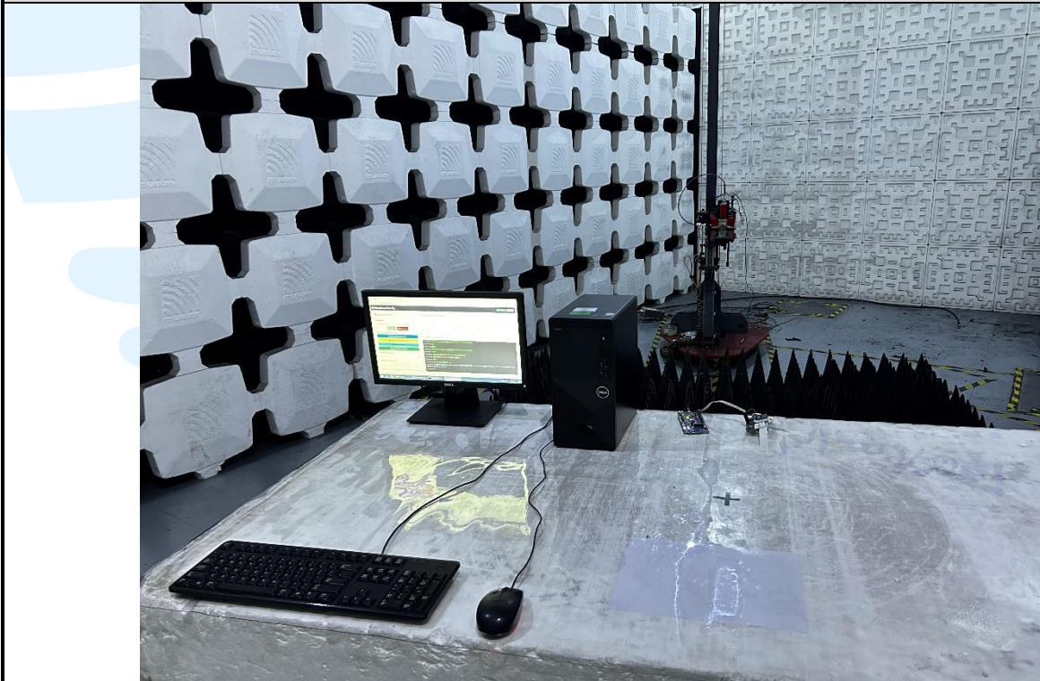
Radiated emission Test Setup-2 (Above 1 GHz)
