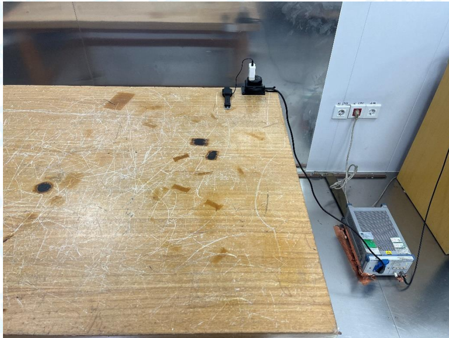
Photo of Setup for Radiated Emission (30MHz~1GHz)
