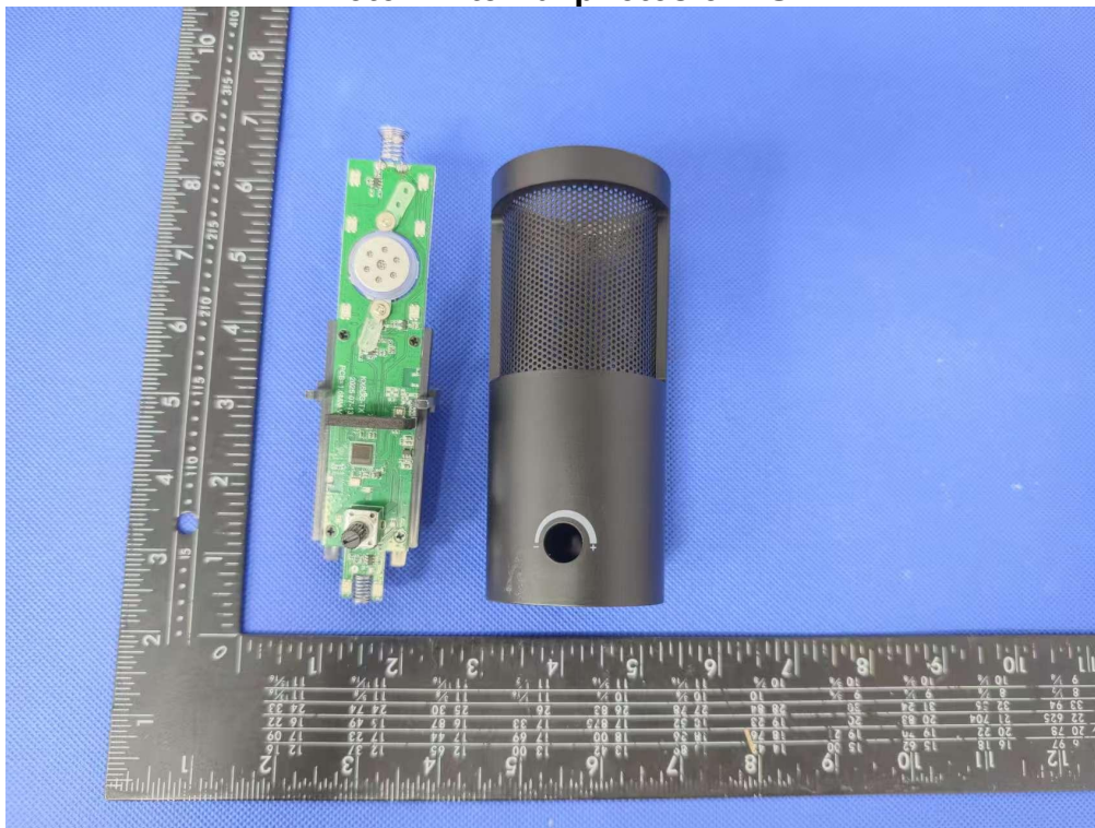
Photo 1 Internal photos of EUT
