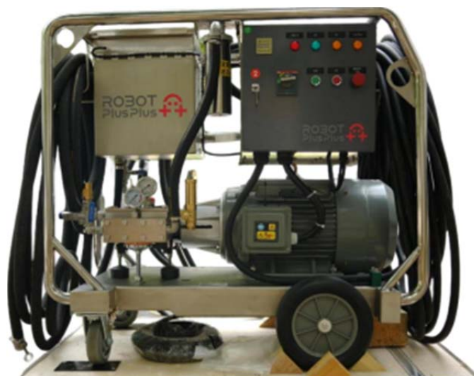
Fig 4.11 High Pressure Water Pump
