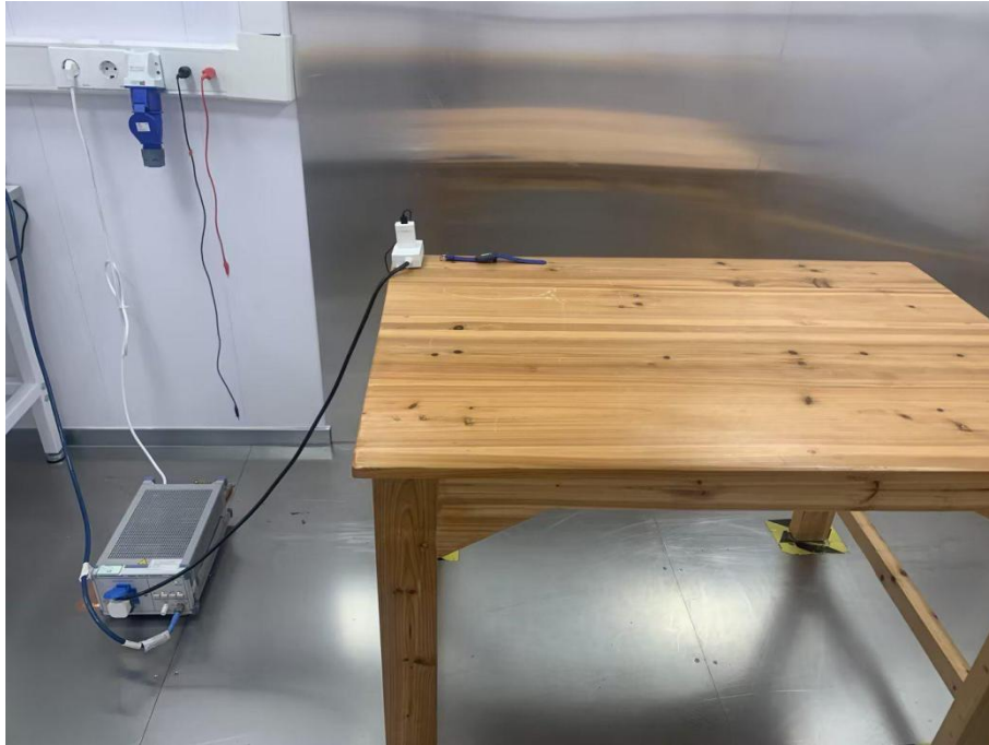
Conducted Emission at AC power line
