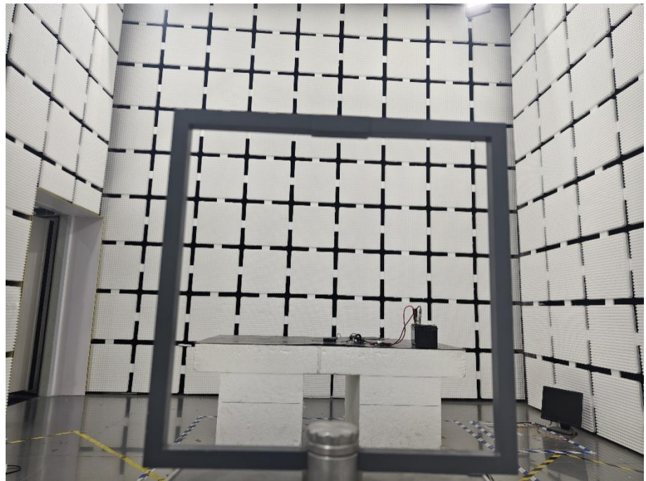
Radiation Emission Test Setup (Below 30MHz)
