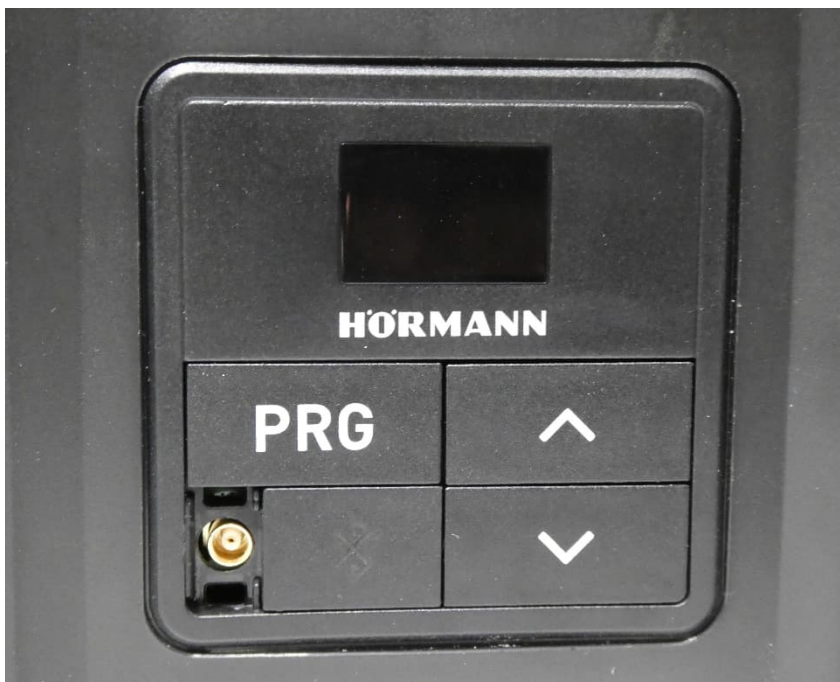
Control unit – cover for external antenna connector removed
