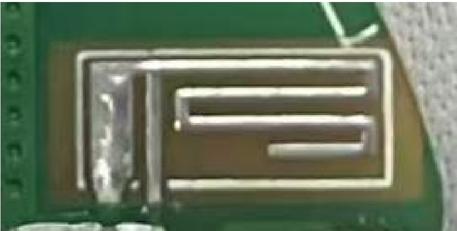
Physical antenna and dimensions
